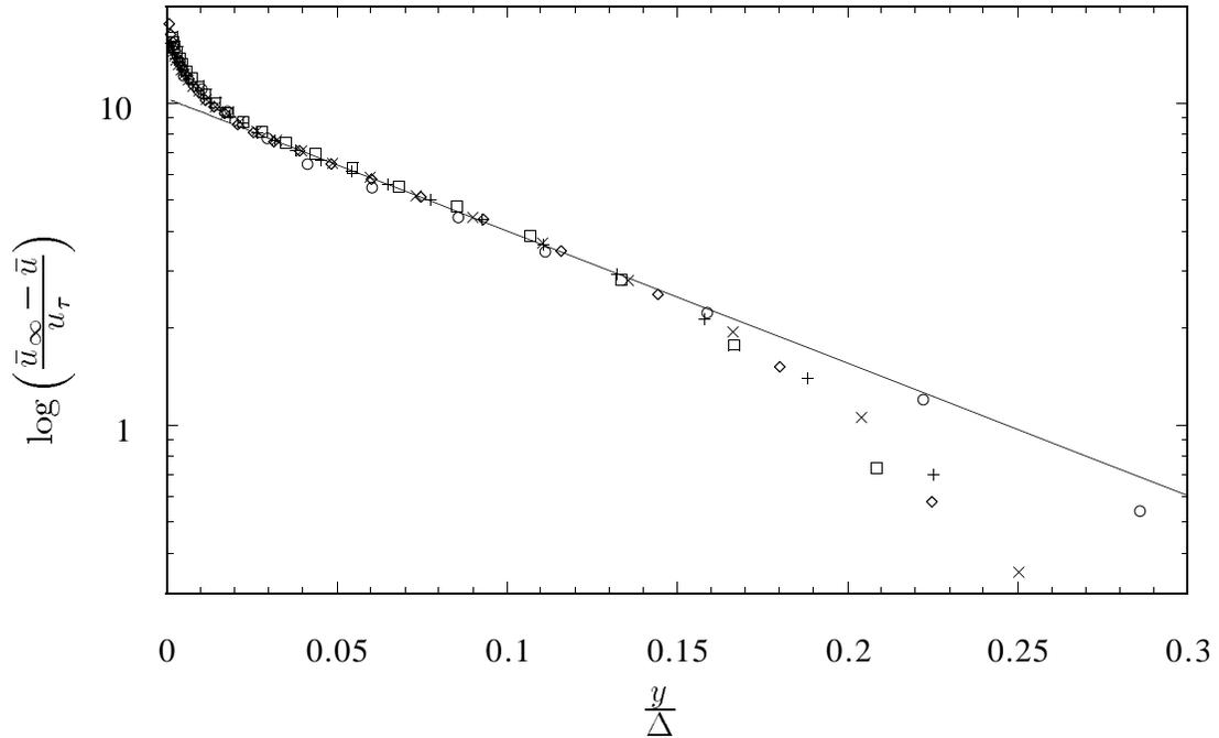
FIGURE 2. Mean velocity of the zero-pressure gradient turbulent boundary layer in lin-log scaling of the defect law:  $\circ$ ,  $Re_\theta = 370000$  (Saddoughi (1994));  $\square$ , and  $\diamond$ ,  $Re_\theta = 60000$  (Fernholz (1995));  $+$ ,  $Re_\theta = 15000$  and  $\times$ ,  $Re_\theta = 20000$  (DeGraaff 1996)); —,  $10.34 \exp(-9.46y/\Delta)$ .
