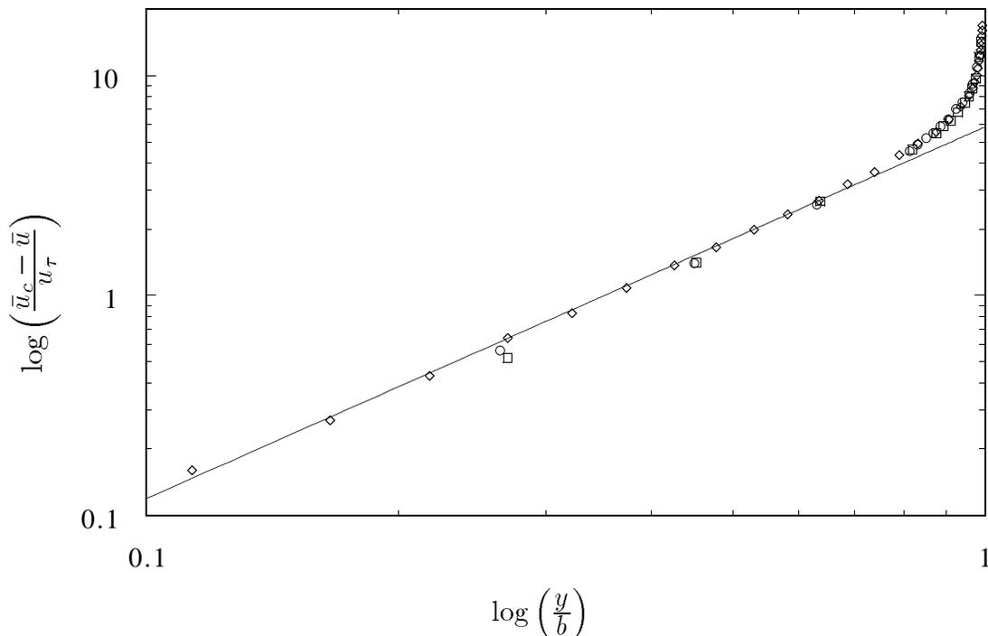
FIGURE 3. Mean velocity of the turbulent channel flow in double-log defect law scaling:  $\circ$ ,  $Re_c = 40000$ ;  $\square$ ,  $Re_c = 23000$  Wei (1989);  $\diamond$ ,  $Re_c = 18000$  Niederschulte (1996); —,  $5.83 (y/b)^{1.69}$ .
