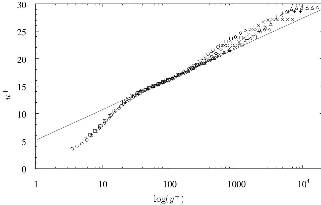
FIGURE 1. Mean velocity of the zero-pressure gradient turbulent boundary layer in log-linear scaling from DeGraaff (1996):  $\circ$ ,  $Re_\theta = 1500$ ;  $\square$ ,  $Re_\theta = 2300$ ;  $\diamond$ ,  $Re_\theta = 3800$ ;  $\times$ ,  $Re_\theta = 8600$ ;  $+$ ,  $Re_\theta = 15000$ ;  $\triangle$ ,  $Re_\theta = 20000$ ; —,  $2.41 \ln(y^+) + 5.1$ .
