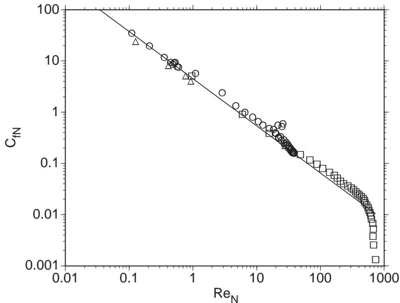
FIGURE 3. Scaling of the magnitude of the skin friction with backflow Reynolds number (see Eq. [5]) in recirculating regions behind a step in Akselvoll & Moin’s (1995)  $Re_h = 28000$  LES:  $\square$  primary,  $\circ$  secondary, and  $\triangle$  tertiary recirculation regions; — Le *et al.*’s (1997) fit from a DNS at  $Re_h = 5100$ . The fall-off at the lower right occurs for points near the head of the main separation bubble at  $x/h \approx 2$ .
