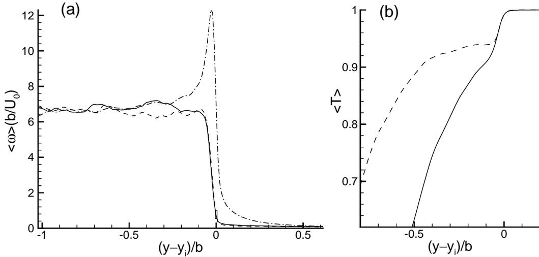
FIGURE 1. Effects of detection parameters on (a) vorticity magnitude, and (b) level of passive scalar, relative to the turbulent/non-turbulent interface. — inner group for  $C_\omega = 0.7U_0/b$ ; ---- outer group for  $C_\omega = 0.7U_0/b$ ; -·-·  $C_\omega = 7U_0/b$
