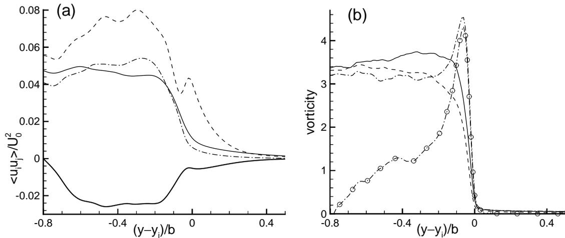
FIGURE 2. Normalized Reynolds stresses and vorticity components for  $C_\omega = 0.7U_0/b$ . (a)  $\langle u^2 \rangle$ ;  $\langle v^2 \rangle$ ;  $\langle w^2 \rangle$ ; lowest curve is  $\langle uv \rangle$ . (b)  $\langle |\omega_x| \rangle$ ;  $\langle |\omega_y| \rangle$ ;  $\langle |\Omega_z| \rangle$ ;  $\cdots \circ \cdots -\langle \Omega_z \rangle$ .
