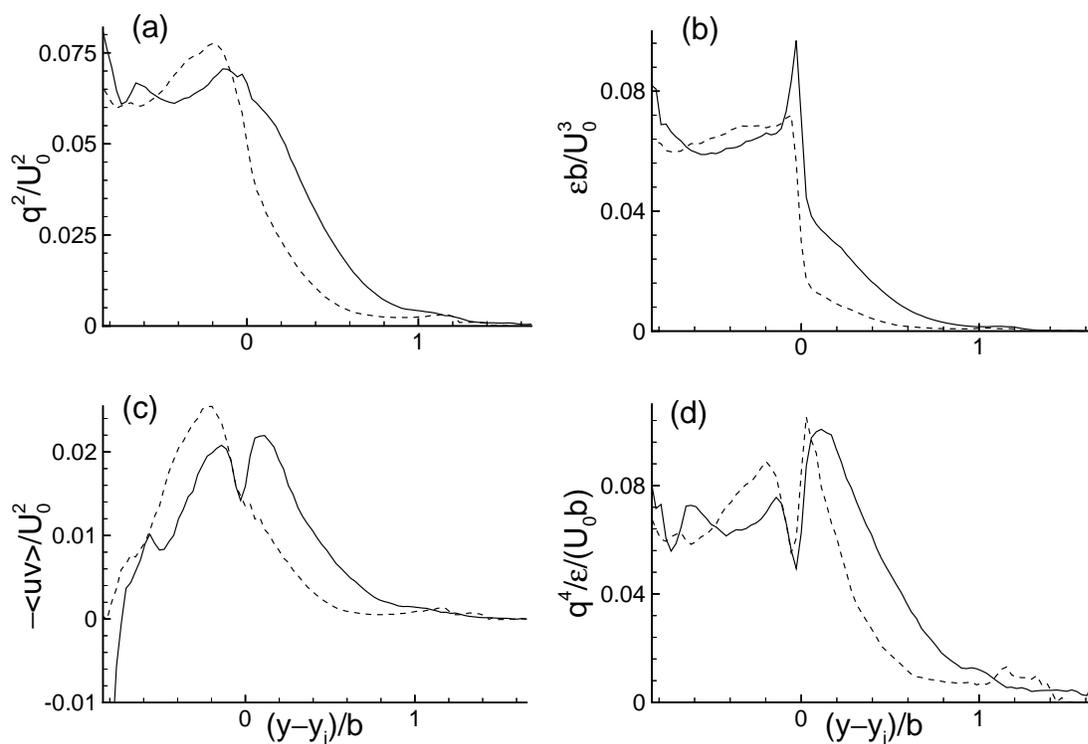
FIGURE A4. Distributions of various conditionally-averaged quantities for threshold values 0.9 (—) and 0.99 (---): a)  $q^2$ ; b)  $\varepsilon$ ; c)  $-\langle uv \rangle$  and d)  $q^4 / \varepsilon$ .
