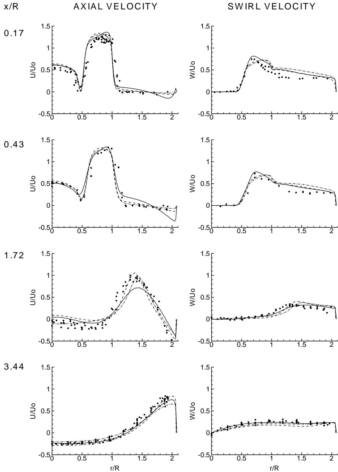
FIGURE 3. Predicted axial and tangential velocity profiles. Symbols: • , exp; — , LES; - - - ,  $k-\epsilon$ ; - · - ,  $v^2 f$ .
