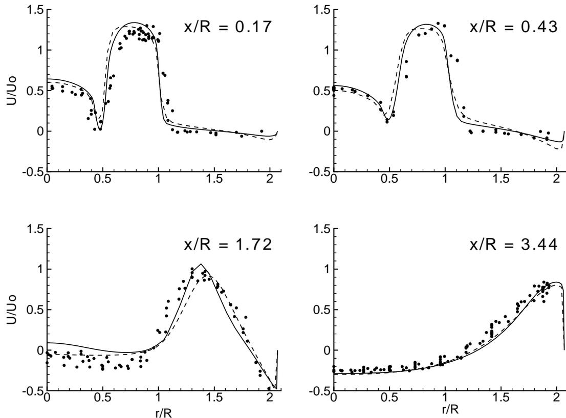
FIGURE 1. Effect of grid density on axial velocity distributions. Symbols:  $\bullet$ , exp; —,  $k\text{-}\epsilon$  126x65; ----,  $k\text{-}\epsilon$  70x40.
