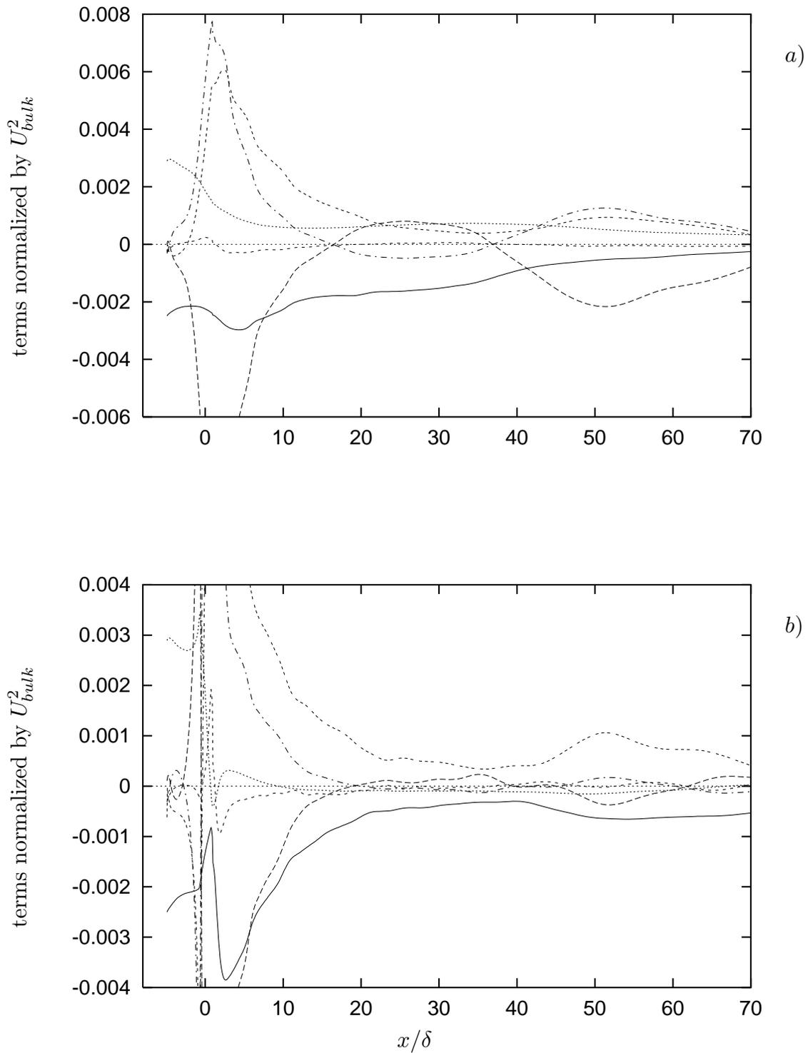
FIGURE 2. Terms of the near wall momentum balance evaluated along flat wall (a) and inclined wall (b) of the diffuser. Line code:  $Adv_x$  ----,  $adv_x$  ----,  $Adv_y$  ---,  $adv_y$  —,  $PG$  ---,  $Visc$  .....
