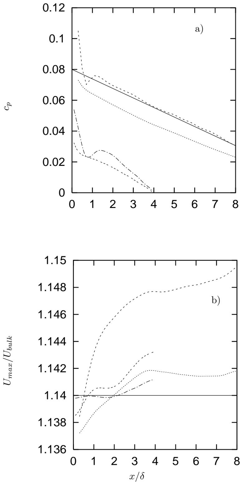
FIGURE 4. Streamwise development of pressure drop (a) and velocity ratio (b) in channel flow using filtered inflow data. Line coding: fine grid LES (target) —, CNM ·····, CWM - - - -, FNM - · - · - ·, FWM — · — ·.
