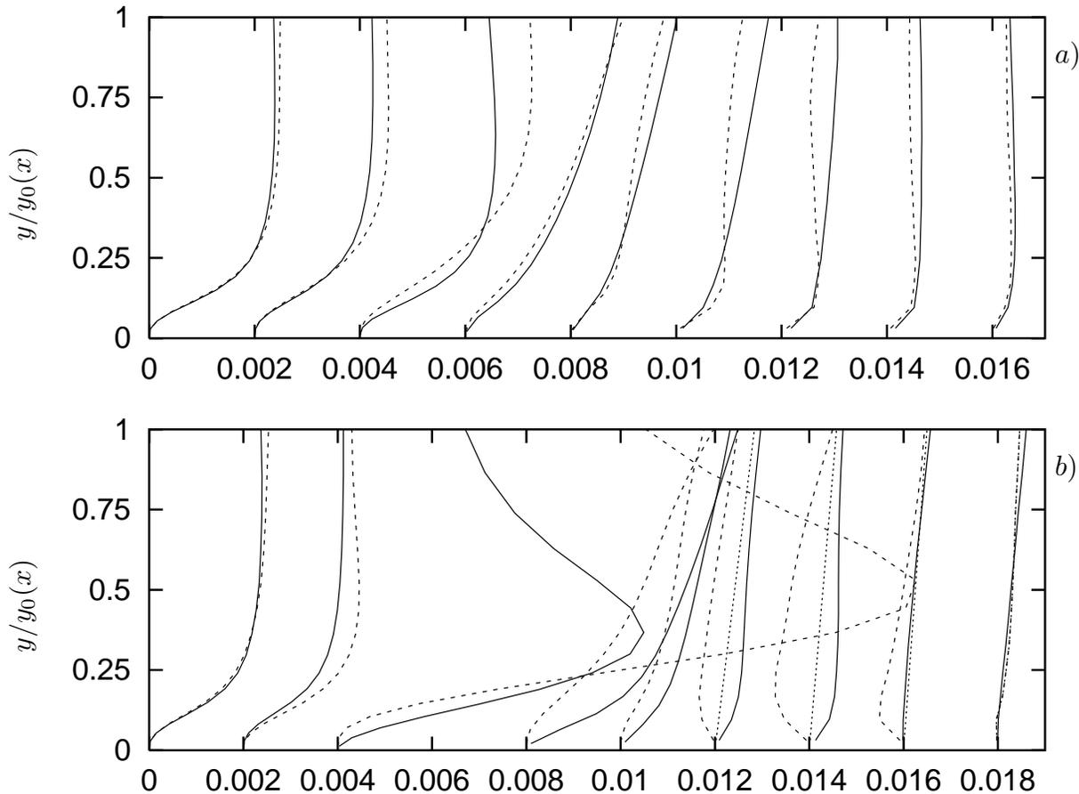
FIGURE 3. Comparison of turbulent shear stress  $|\overline{uv} + \tau_{SGS}|$  from fine-grid LES — with prediction from the Johnson-King model  $\nu_t dU/dy$  ---- and a linear extrapolation  $\overline{uv}_{max} y/y_{max}$  ..... at stations  $x/\delta = -4.1, -1.0, 1.0, 6.3, 14.2, 26.4, 38.1, 45.6, 65.8$  along flat (a) and inclined wall (b). The distance from the wall has been normalized with the thickness  $y_0$  of the near-wall zone.
