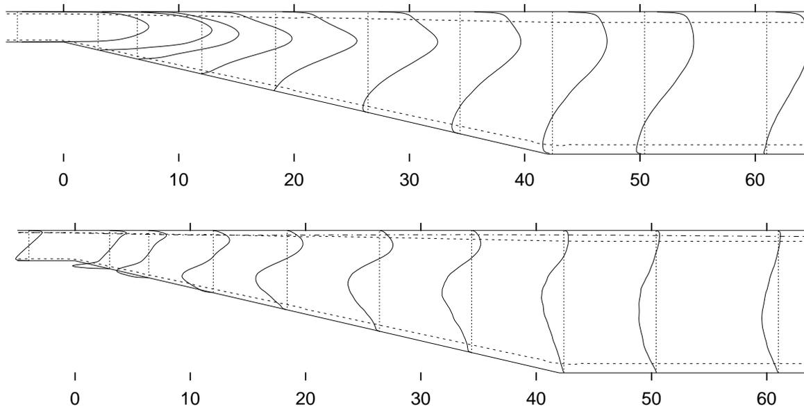
FIGURE 1. Profiles of mean streamwise velocity component (*top*) and shear stress  $\overline{uv}$  (*bottom*) at stations  $x/\delta = -4, 3, 6.4, 12, 18.4, 26.4, 34.4, 42.4, 50.4, 61$ . The dashed lines mark the border of the near wall zone defined to be 7% of the local duct height, whereas the dash-dotted line corresponds to a distance of 70 wall units.
