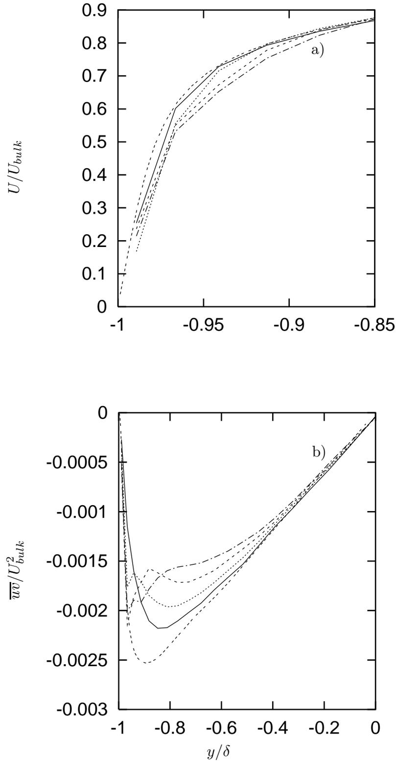
FIGURE 5. Profiles of  $\overline{U}(y)$  (a) and  $\overline{wv}$  (b) from case FWM at distances  $x/\delta = 0.2$  —, 0.8 ·····, 2. ----, 3.4 -·-·-. Profiles from the fine-grid LES are marked as - - - - .
