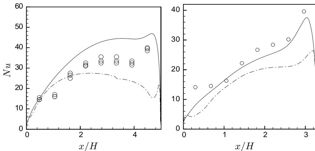
FIGURE 11. Nusselt number distribution on the floor for  $d/w = 0.1$  (left) and  $d/w = 0.2$  (right). —  $v^2 - f$ , ---  $k - \epsilon$ ,  $\circ$  experimental data of Metzger *et al.* (1989). The experiment was repeated with three different inlet temperatures and all measured data sets are shown in this figure.
