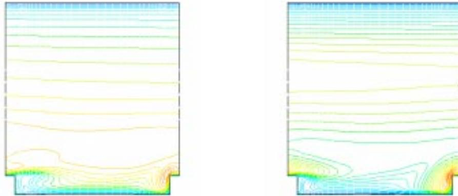
FIGURE 8. Nusselt number contours on the smooth side wall of the computational domain computed using  $v^2 - f$  turbulence model (contour level is 0.3–2.0) (left) and  $k - \epsilon$  turbulence model (contour level is 0.3–2.2) (right).
