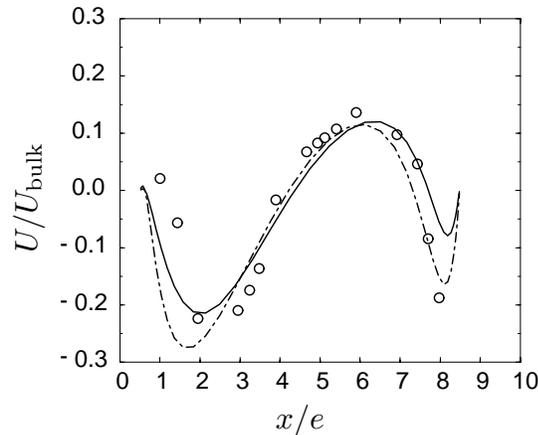
FIGURE 4. Comparison of the streamwise velocity component,  $U$ , at  $y/e = 0.1$  on the symmetry plane of the computational domain. This figure shows data from a 1s simulation with  $p/e = 9$ . —  $v^2 - f$  turbulence model, ---  $k - \epsilon$  2 layer model,  $\circ$  experimental data of Rau *et al.* (1998).
