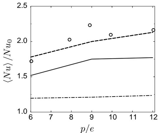
FIGURE 7. Average Nusselt number on the floor of the computational domain. —  $v^2 - f$ , ----  $v^2 - f$  for “reduced” domain, -.-  $k - \epsilon$ ,  $\circ$  experimental data from Rau *et al.* (1998).
