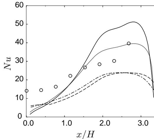
FIGURE 12. Nusselt number distribution on the floor for  $d/w = 0.2$ . Calculations performed with  $k - \epsilon$  model with standard wall functions.—  $y^+ \simeq 3$ , .....  $y^+ \simeq 5$ , ———  $y^+ \simeq 30$ , - - -  $y^+ \simeq 50$ ,  $\circ$  experimental data of Metzger *et al.* (1989).
