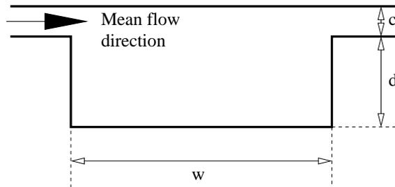
FIGURE 2. Two-dimensional computational domain for blade tip simulations.
