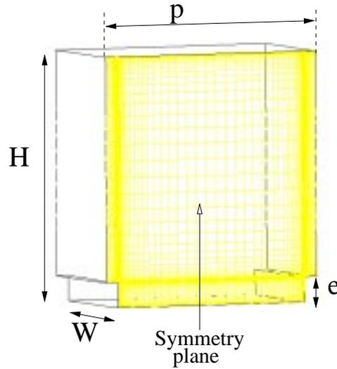
FIGURE 1. Three-dimensional computational domain for ribbed passage simulations.
