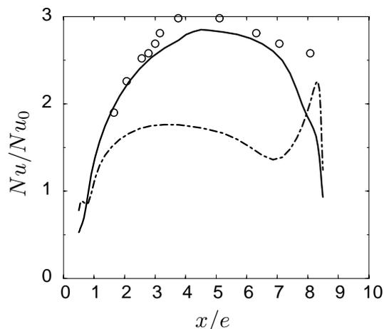
FIGURE 5. Comparison of the Nusselt number distribution for the 2-sided ribbed channel with  $p/e = 9$  on the symmetry plane of the computational domain. —  $v^2 - f$  turbulence model, ---  $k - \epsilon$  2 layer model,  $\circ$  experimental data of Rau *et al.* (1998).
