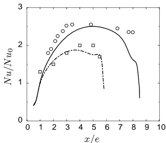
FIGURE 6. Nusselt number distribution on the floor of the symmetry plane. —  $v^2 - f$  with  $p/e = 9$ ,  $\circ$  corresponding experimental data from Rau *et al.* (1998), ---  $v^2 - f$  with  $p/e = 6$ ,  $\square$  corresponding experimental data from Rau *et al.* (1998).
