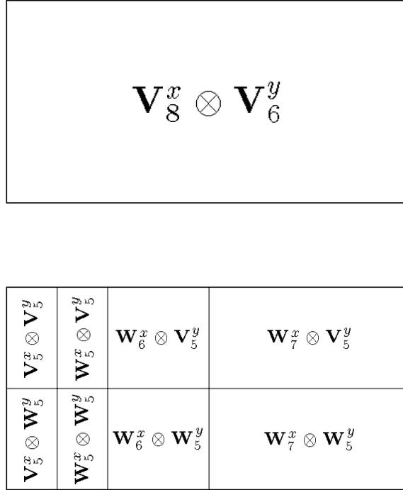
FIGURE 1. 2D tensor decomposition of initial computational domain into wavelet subspaces.
