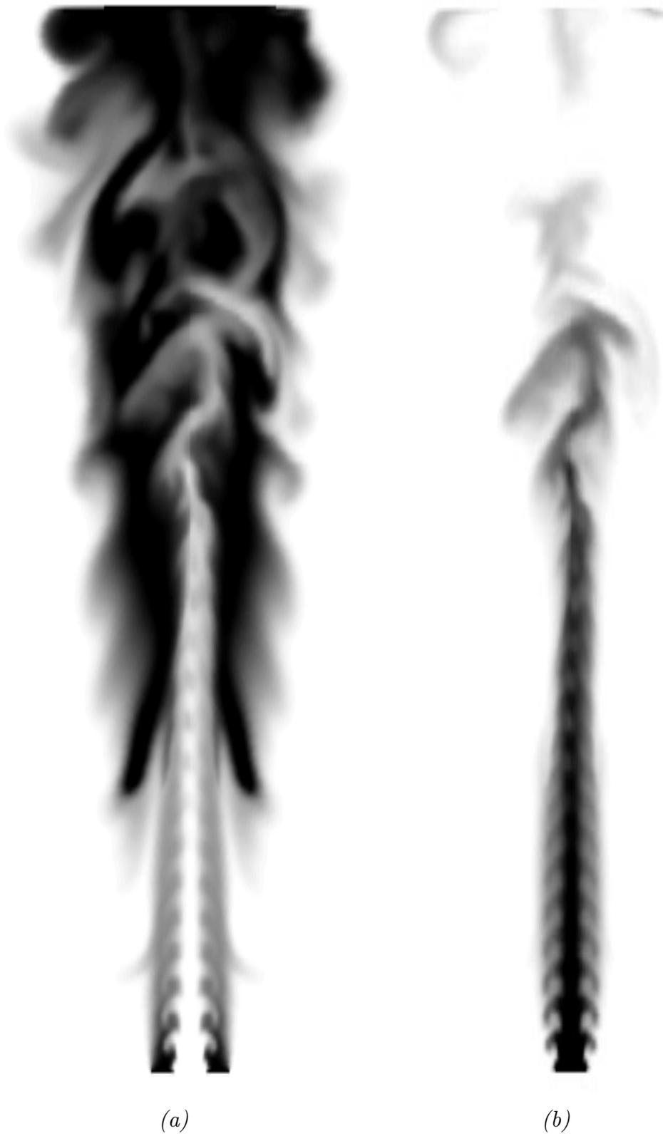
FIGURE 3. Results of LES of piloted jet flame: (a) non-dimensional temperature: white-black,  $T/T_0 = 1$  to 5; (b) mass fraction of fuel: white-black,  $Y_F = 0$  to 1.
