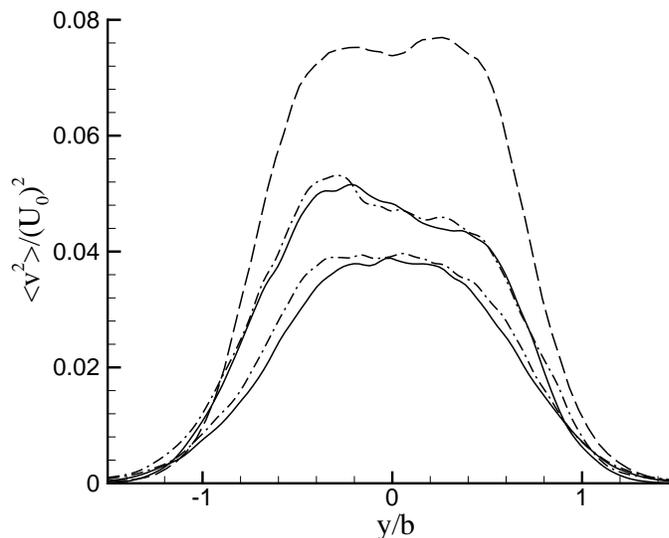
FIGURE 1. Distributions of  $\langle v^2 \rangle$  from spectral (---) and AGE (—) DNS at  $\tau = 42.8$  (lowest curves) and  $\tau = 91.5$  (middle curves). The uppermost curve is  $\langle v^2 \rangle$  at  $\tau = 74.4$  from the top-hat initial profile.
