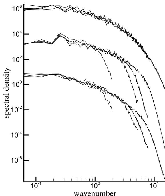
FIGURE 4. Streamwise power spectra on the centerplane at  $\tau = 91.5$  for  $u$  (bottom),  $v$  (middle), and pressure (top) from AGE DNS and auto-LES. From left to right by rolloff point, the grids used were R8, R3, R2, and DNS.
