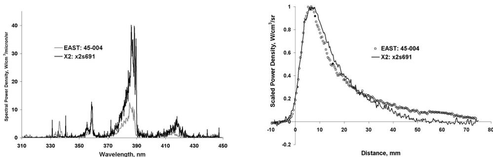
FIGURE 8. Experimental results obtained by means of the X2 (University of Queensland) and EAST (NASA Ames Research Center) facilities for 5.7 km/s velocity, 13 Pa pressure, 98% $N_2$  and 2% $CH_4$ . Left: peak spectral power density; right: scaled power density integrated over 310 – 450nm.
