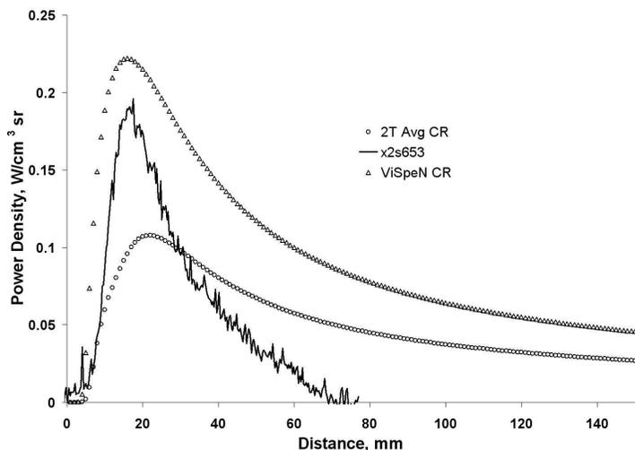
FIGURE 9. Comparison of computational models and X2 experiment (unbroken line) for 5.15 km/s velocity, 13 Pa pressure, 98% $N_2$  and 2% $CH_4$ . Vibrational CR model ViSpeN (triangles), multi-temperature CR model (circles).
