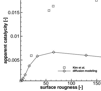
FIGURE 6. Apparent catalytic activity versus surface roughness for a 2-D cavity. The intrinsic catalytic activity is set to  $2.5 \times 10^{-4}$  at the cavity walls, the cavity width is set to  $1 \times 10^{-6} \text{ m}$  and the cavity depth is varied in order to obtain the relevant surface roughness, which is computed as the ratio of the wetted surface to the geometrical surface:  $R = (2 \times L_2 + L_1)/L_1$ .
