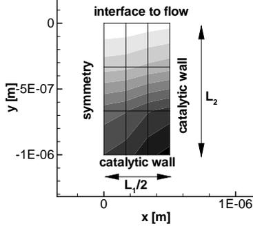
FIGURE 5. The computational domain, the grid, boundary conditions and the solution in terms of concentration of atomic nitrogen. The inlet concentration of N is  $0.1 \times 3.25 \times 10^{-3} \text{ mol/m}^3$  and of  $N_2$  equals  $0.9 \times 3.25 \times 10^{-3} \text{ mol/m}^3$ . A recombination coefficient boundary condition has been used with  $\gamma = 1$ .
