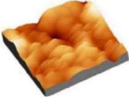
FIGURE 2. Atomic force microscopy photograph of a silicon carbide surface after plasma exposure at the VKI Plasmatron. The size of the slab is  $10 \times 10 \times 1\mu\text{m}$  (Verant *et al.* 2006).
