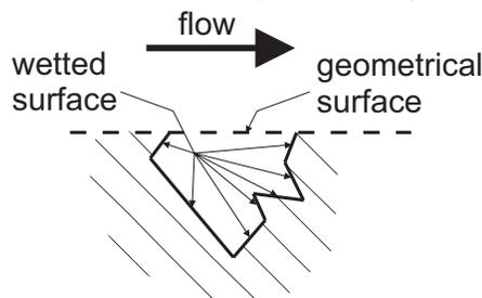
FIGURE 1. Schematic of a surface roughness feature. The actual "wetted" surface on which the catalysis phenomenon takes place can be significantly larger than the geometrical surface seen by an observer.
