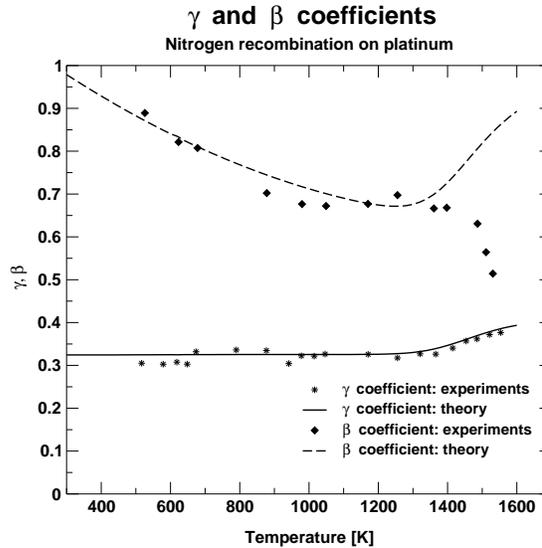
FIGURE 9.  $\gamma$  and  $\beta$  coefficients for nitrogen recombination on platinum.
