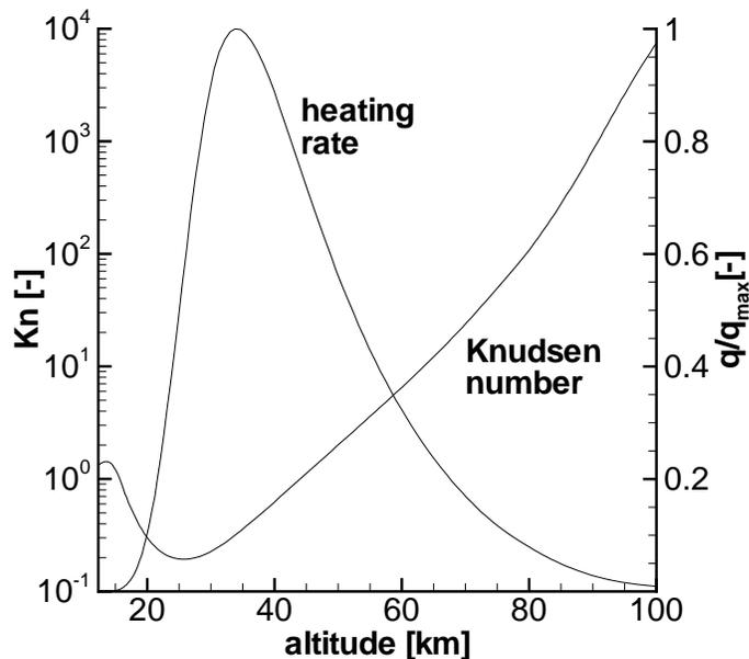
FIGURE 4. Knudsen number and normalized heating rate for the predicted flight trajectory of the EXPERT capsule. The Knudsen number is based on a roughness feature dimension of  $1 \times 10^{-6} m$  and a mean free path (Moore 1972) computed from the expected stagnation pressure based on the DKR formula (Detra *et al.* 1957) and the diameter of the nitrogen molecule (Moore 1972).
