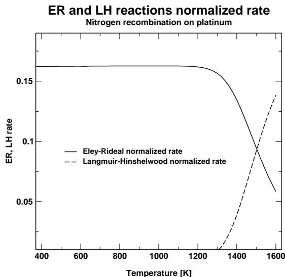
FIGURE 8. ER and LH normalized rate for nitrogen recombination on platinum.
