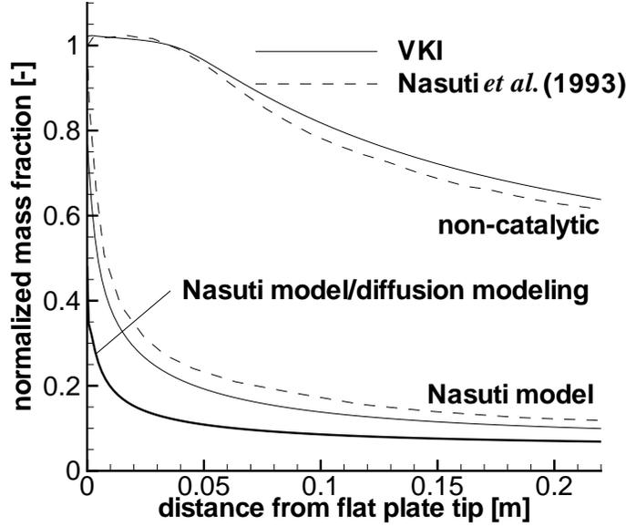
FIGURE 7. Normalized oxygen mass fraction at the wall for chemical non-equilibrium flat plate flow. The inlet conditions and boundary conditions of Nasuti *et al.* (1993) are applied.
