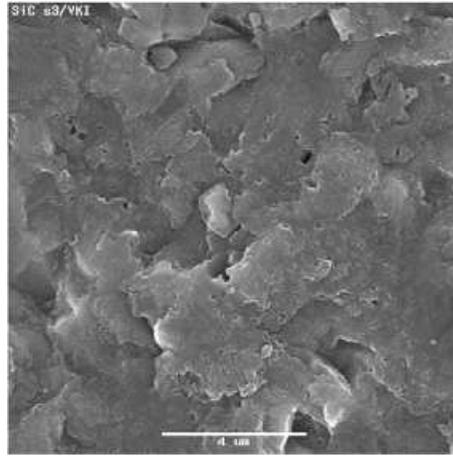
FIGURE 3. Scanning electron microscopy photograph of a silicon carbide surface after plasma exposure at the VKI Plasmatron (Verant *et al.* 2006). The size of the photograph is  $12 \times 12\mu\text{m}$ .
