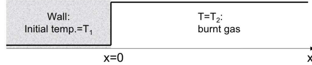
FIGURE 3. The IFF (Infinitely Fast Flame) limit. Solid line: initial temperature profile.
