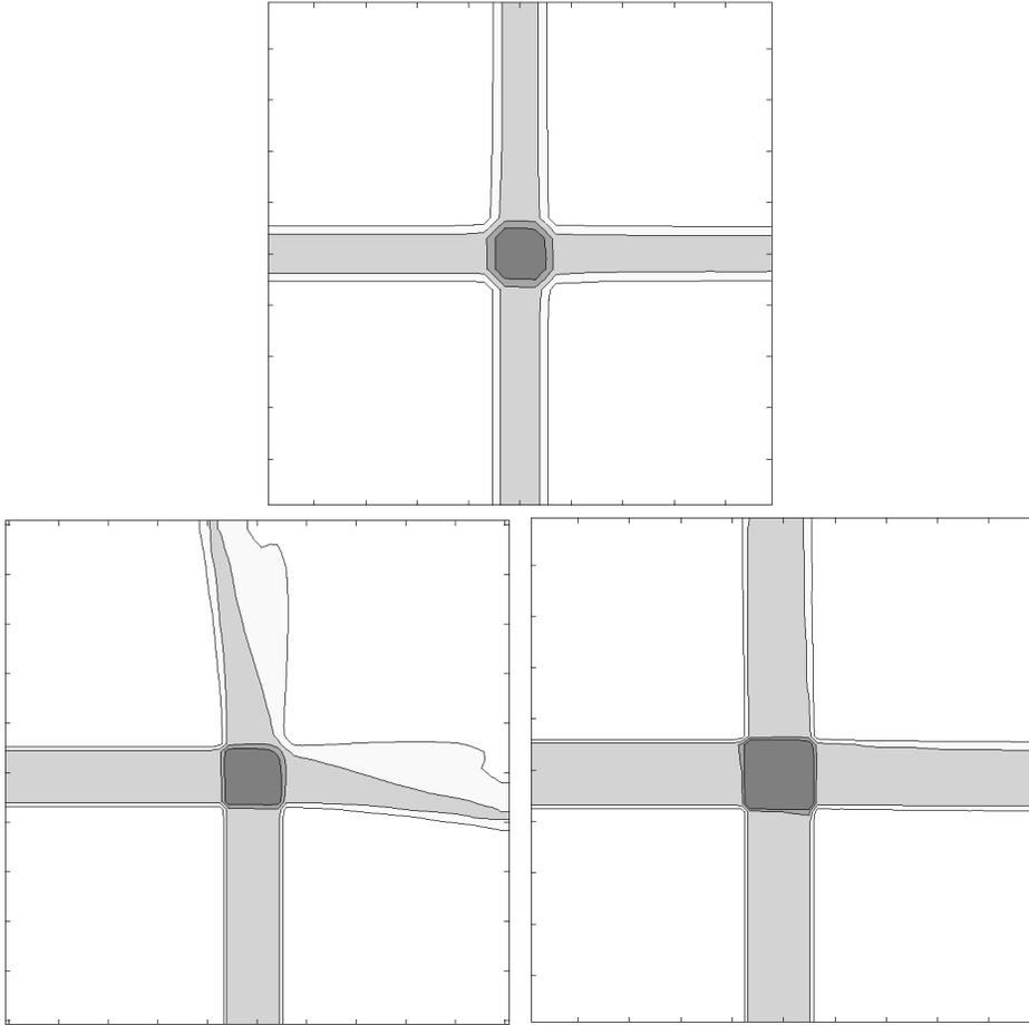
FIGURE 4. Particles' number density map and isocontours for crossing jets with  $Kn = 5$ . Density proportional to darkness. Domain size:  $1 \text{ m} \times 1 \text{ m}$ . Top left: Lagrangian. Top right: full second-order model. Bottom left: QMOM #1. Bottom right: QMOM #2.
