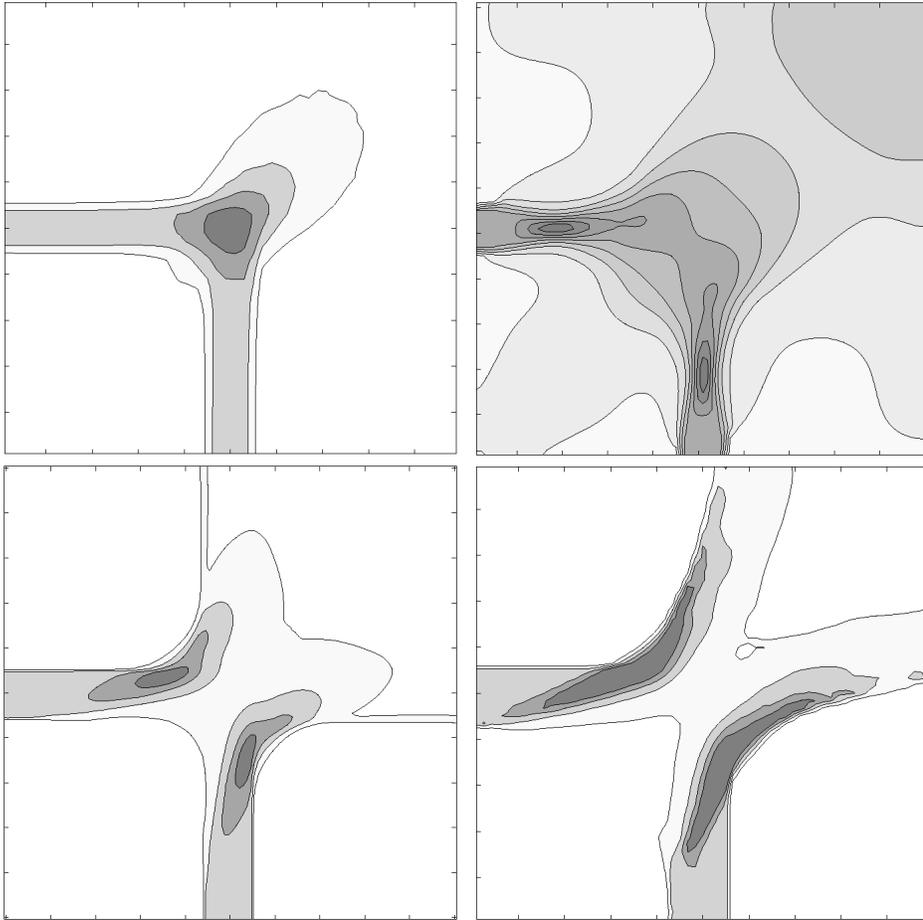
FIGURE 2. Particles' number density map and isocontours for crossing jets with  $Kn = 0.1$ . Density proportional to darkness. Domain size:  $1 \text{ m} \times 1 \text{ m}$ . Top left: Lagrangian. Top right: full second-order model. Bottom left: QMOM #1. Bottom right: QMOM #2.
