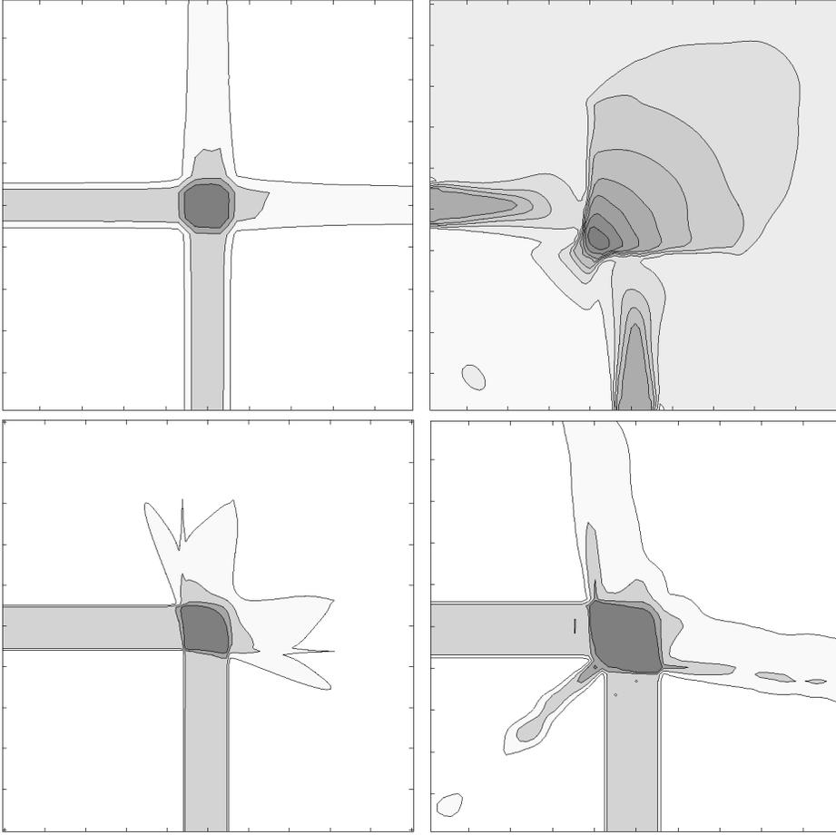
FIGURE 3. Particles' number density map and isocontours for crossing jets with  $Kn = 1$ . Density proportional to darkness. Domain size:  $1 \text{ m} \times 1 \text{ m}$ . Top left: Lagrangian. Top right: full second-order model. Bottom left: QMOM #1. Bottom right: QMOM #2.
