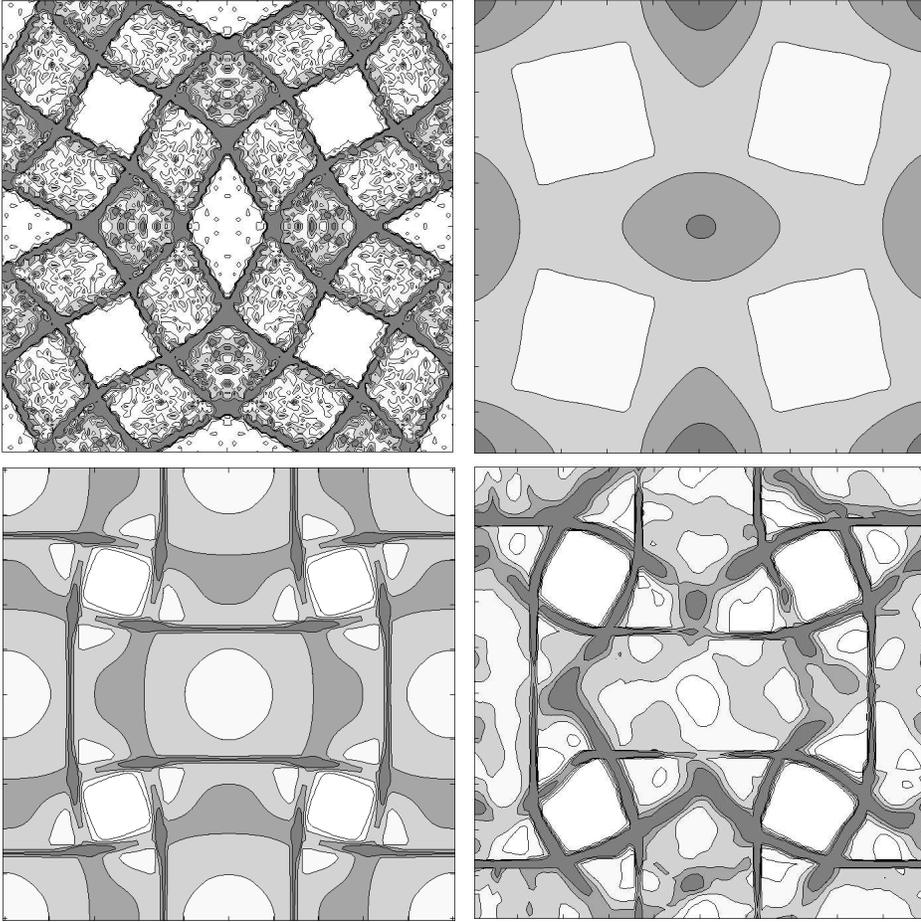
FIGURE 5. Particles' number density map and isocontours for Taylor-Green flow, stationary state,  $St = 1$ . Density proportional to darkness. Domain size:  $1\text{ m} \times 1\text{ m}$ . Top left: Lagrangian. Top right: full second-order model. Bottom left: QMOM #1. Bottom right: QMOM #2.
