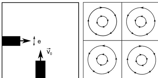
FIGURE 1. Schematics showing the two test cases. Left: crossing jets. Right: Taylor-Green flow.
