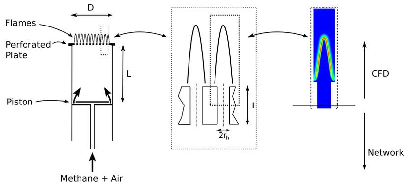
FIGURE 2. Sketch of the burner test rig with details of the perforated-plate geometry (middle) and CFD domain (right).
