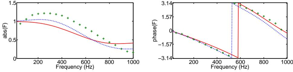
FIGURE 9. Amplitude (left) and phase (right) of the flame transfer functions  $F(\omega)$ : Computational results obtained with adiabatic (red, solid line) and isothermal (350 K) (blue, dashed line) wall at the front of the plate vs. experimental data of Noiray *et al.* 2007 (+, green). The sign of the phase has been changed to match the sign convention of this work.
