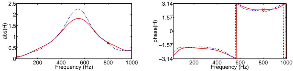
FIGURE 10. Comparison of amplitude (left) and phase (right) of the frequency response function  $H$  for an adiabatic (red, solid) and isothermal (350 K) (blue, dashed) wall at the front of the plate. The red “X” marks the result of single frequency harmonic forcing for the adiabatic case.
