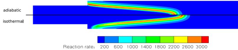
FIGURE 8. Comparison of the position of the flame (reaction rate) for an adiabatic (top) and isothermal (350K) (bottom) wall at the front of the plate
