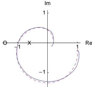
FIGURE 5. Polar plot of flame-transfer function  $F(\omega)$ .
