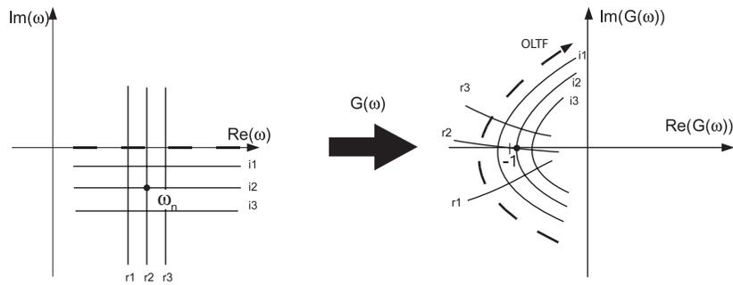
FIGURE 3. The Nyquist curve (dotted line in the right plot) is the image of the positive half of the real axis in the  $\omega$ -plane under the OLTf mapping  $\omega \rightarrow G(\omega)$ . Case shown corresponds to an unstable eigenfrequency with  $\Im(\omega) < 0$ .
