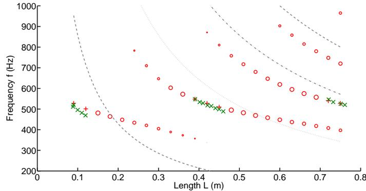
FIGURE 11. Stability map of the perforated plate burner (“Plate 4” with  $l = 30$  mm): frequencies and growth rates of the first four eigenmodes vs. plenum length. Unstable modes observed in experimental values: “x”, CNN from isothermal calculation with  $T_W = 350$  K and pressure-loss coefficient  $\zeta = 42$ : “o” for stable, “+” for unstable modes. The size of the marker indicates the magnitude of the growth/decay rate. Dashed lines correspond to the first quarter-wave modes of the plenum.
