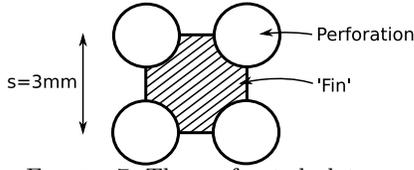
FIGURE 7. The perforated plate as “cooling fin”.
