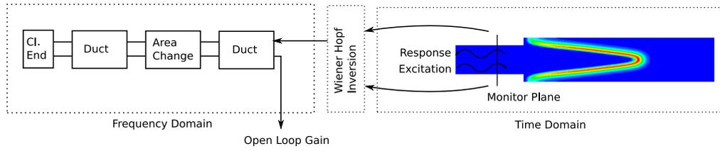
FIGURE 4. Coupling between network model and CFD using correlation analysis
