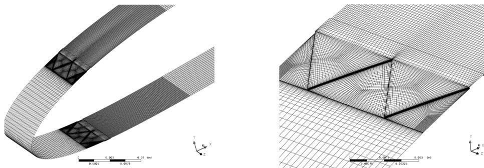
FIGURE 3. Left: Grid refinement on the airfoil for resolving the boundary-layer transition process. Right: Close-up view on the boundary-layer trip mesh region.
