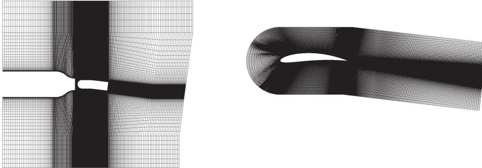
FIGURE 2. Left: Grid topology of the wind tunnel setup in Siegen for initial RANS computations. Right: LES truncated domain, extracted from the full wind tunnel setup.
