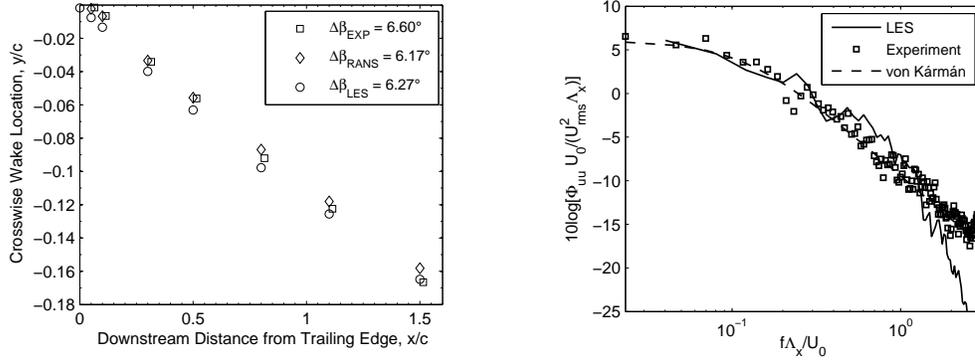
FIGURE 10. Mean and fluctuating velocities in the wake. Left: Mean flow deflection. Right: Streamwise velocity spectra.
