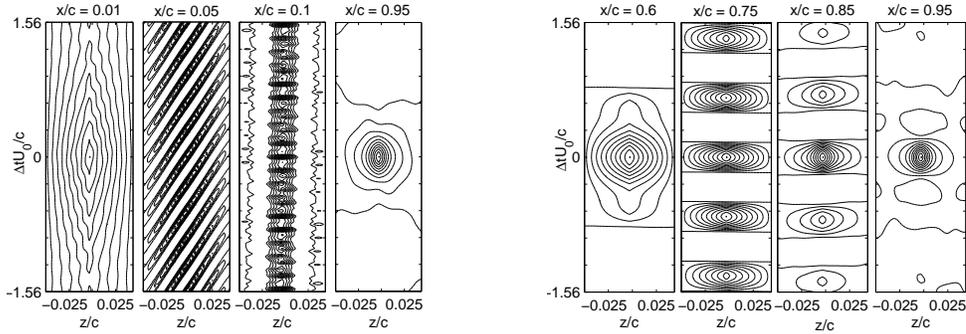
FIGURE 7. Space-time correlation of wall-pressure fluctuations at various  $x/c$  locations. Left: Pressure side. Right: Suction side. Contour values are from 0 to 0.9 with increment 0.1.
