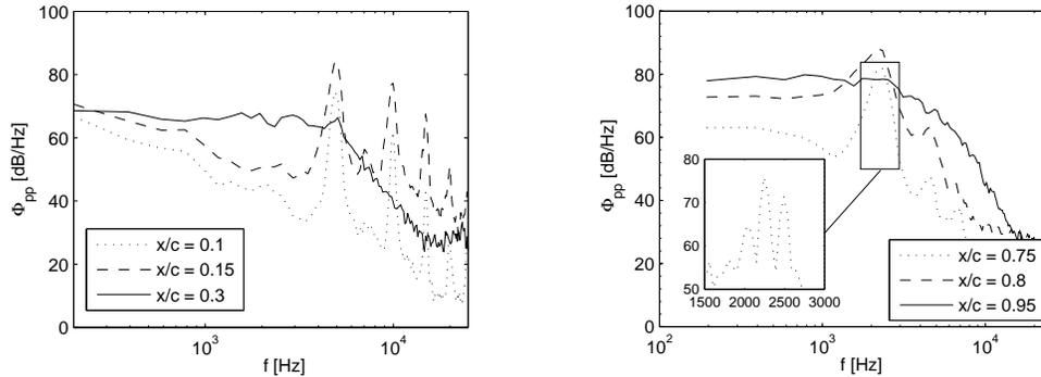
FIGURE 6. Wall-pressure spectra with reference to  $2 \times 10^{-5} Pa$ , at selected  $x/c$  locations. Left: Pressure side. Right: Suction side. The zoom window shows the broad spectral peak with higher resolution.
