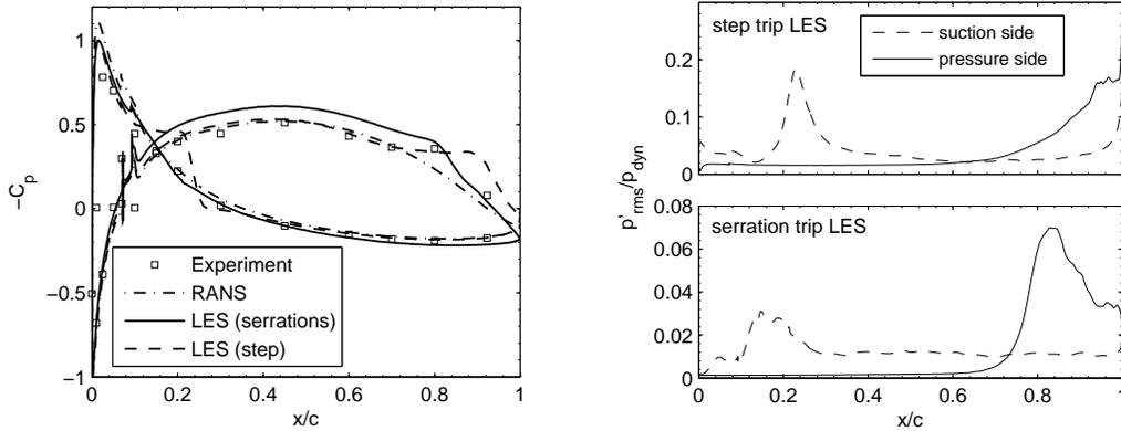
FIGURE 4. Left: Mean wall-pressure coefficient  $-C_p$  on the airfoil. Right: root mean squared (rms) values of the pressure fluctuations along the chord for the step trip LES and the serration trip LES.
