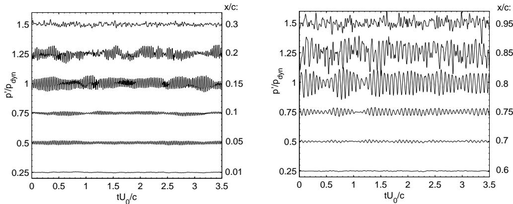
FIGURE 5. Airfoil wall-pressure fluctuations at different  $x/c$  locations. Left: Pressure side. Right: Suction side. Fluctuations are centered around artificial vertical offsets 0.25, 0.5, ..., 1.5.
