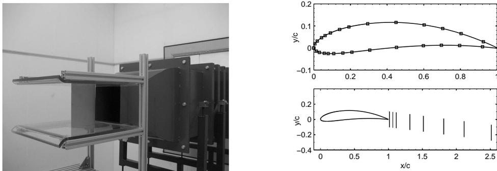
FIGURE 1. Left: Experimental setup in front of the wind tunnel at the University of Siegen. Right: Locations for lift measurements on the NACA6512-63 airfoil (top) and wake velocity measurements (bottom).
