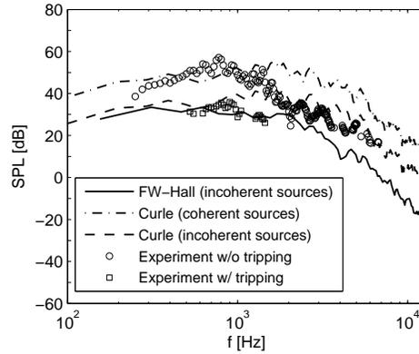
FIGURE 11. Sound-pressure levels in dB with  $\Delta f = 3.125 \text{ Hz}$  and reference to  $2 \times 10^{-5} \text{ Pa}$ . Predictions are from the serrated trip LES.
