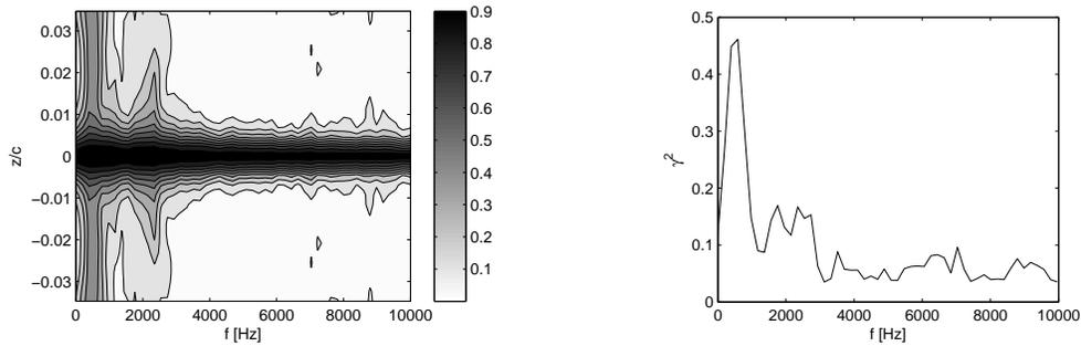
FIGURE 8. Pressure fluctuations at  $0.95 c$  on the suction side. Left: Isochorence values. Right: Variation of coherence with frequency for  $\Delta z/c = 0.0278$ .
