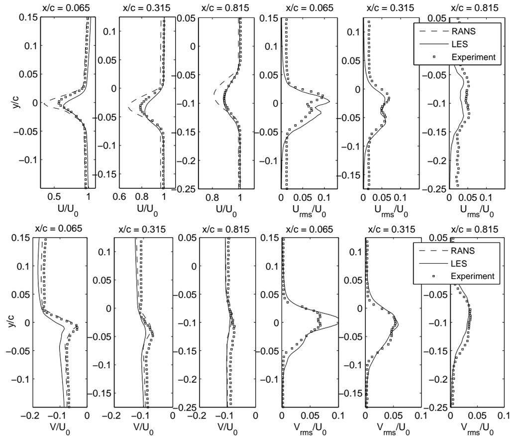
FIGURE 9. Normalized wake velocity data at three  $x/c$  locations. Top: Streamwise mean and rms velocity  $U/U_0$  and  $U_{rms}/U_0$ . Bottom: Crosswise mean and rms velocity  $V/U_0$  and  $V_{rms}/U_0$ .
