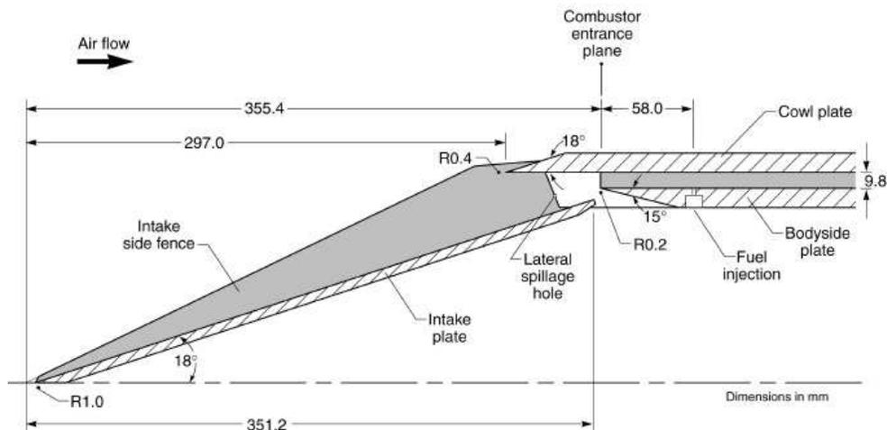
FIGURE 1. The geometry of the nose and the combustor inlet of the HyShot hypersonic vehicle (Smart *et al.* 2006). Note that the vehicle is symmetric with two identical combustion chambers, but the fuel was injected only in one.
