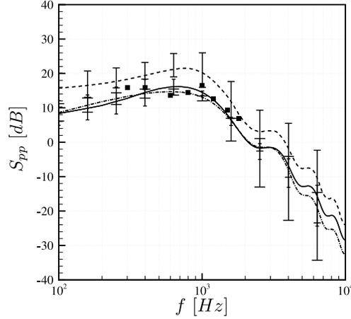
FIGURE 7. Means and uncertainty bars of far-field acoustic spectra for the different methods, in the mid-span plane above the airfoil ( $\theta = 90^\circ$ ) at  $R = 2$  m from the trailing edge. (Dash-dot and large uncertainty bars) Rozenberg's model, (plain and small uncertainty bars) Panton & Linerbarger's model, (dash and medium uncertainty bar) LES. (Square) Experiments.
