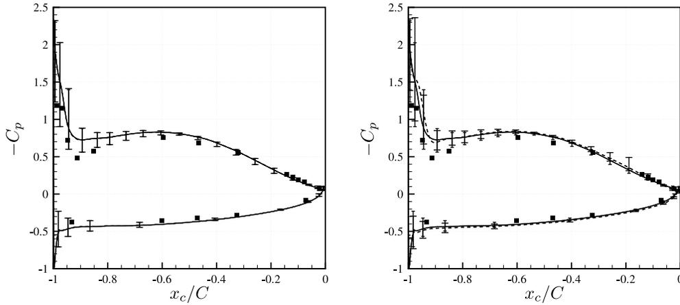
FIGURE 4. Mean wall-pressure coefficient  $C_p$  and corresponding uncertainty bars. (Left) Comparison of RANS UQ-based methods: (plain line and small uncertainty bars) SC and (dashed line and large uncertainty bars) MC. (Right) Comparison of flow prediction method using SC: (plain line and small uncertainty bars) RANS computations and (dashed line and large uncertainty bars) LES computations. (Square) Experiments.
