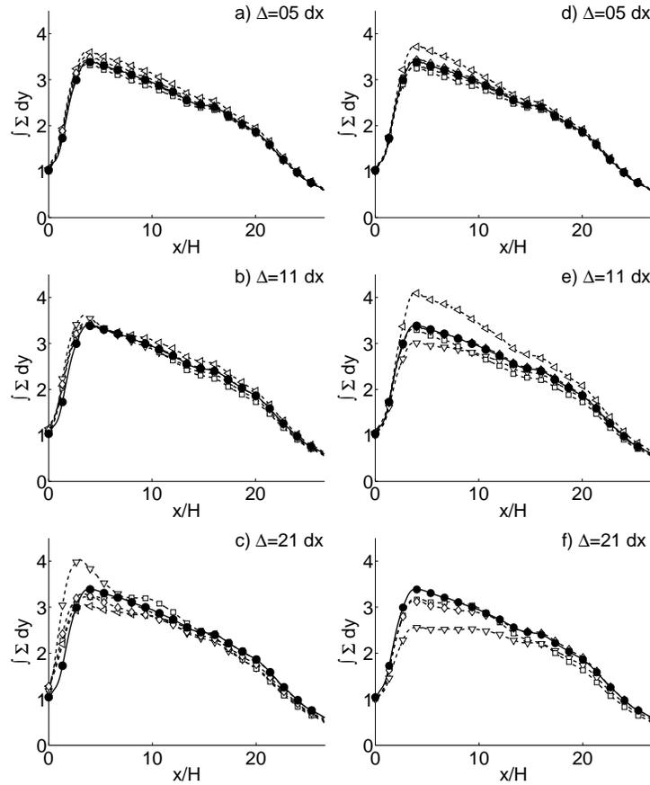
FIGURE 2.  $\int \Sigma dy$ , for DNS and models. Left : Constant coefficients; Right : Dynamic coefficients. Legend: ( $\bullet$ ) DNS; ( $\diamond$ ) Proposed model; ( $\triangleright$ ) Pitsch; ( $\nabla$ ) Colin ( $\square$ ) Charlette
