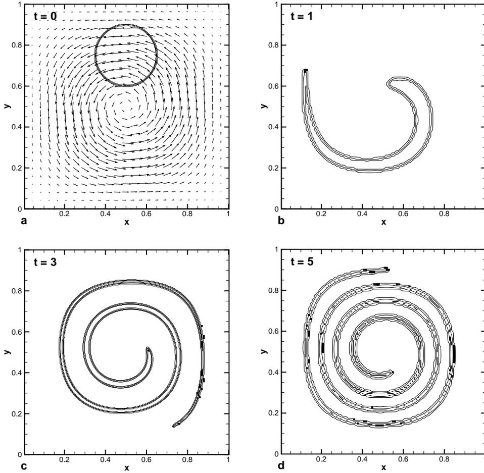
FIGURE 2. Results of interface deformation in the single vortex flow using a two-scale grid system ( $\Delta = 0.01$ ,  $r = 3$ , volume fraction contours of  $\alpha = 0.05, 0.5$  and  $0.95$  obtained from level sets on the coarse grid): (a) initial interface location and velocity field, (b), (c) and (d) cells with unresolved interface (black squares) at time  $t = 1, 3, 5$ .
