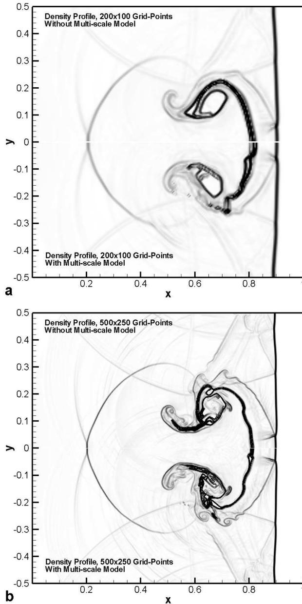
FIGURE 3. Comparison of the results of the shock-bubble interaction problem at time  $t = 0.2$ : Schlieren-type images (mirrored images from symmetric axes are results with a multi-scale model) of density for (a)  $\Delta = 5 \times 10^{-3}$ , and (b)  $\Delta = 2 \times 10^{-3}$ .
