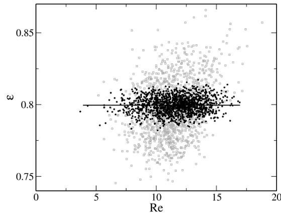
FIGURE 6. Scatter plot of the gas volume fraction and Reynolds number experienced by free-falling spheres for different filter sizes:  $\Delta = 15d_p$  (line),  $7.5d_p$  (black dots), and  $3.75d_p$  (grey squares).
