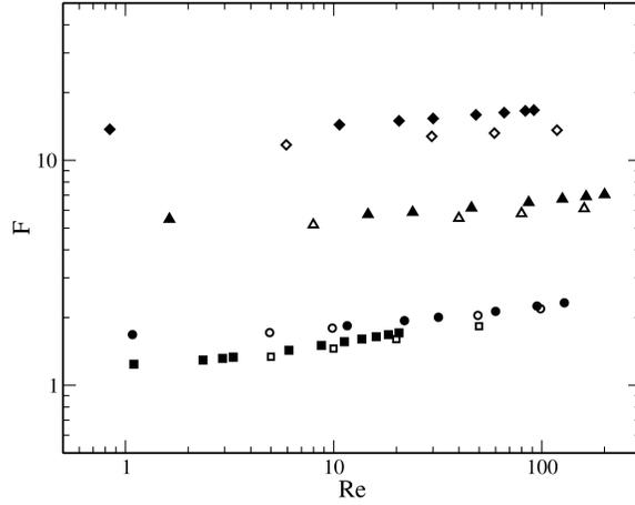
FIGURE 3. Non-dimensional drag force as function of the particle Reynolds number for simple cubic arrangements of spheres. Comparison between Hill *et al.* (2001) (filled symbols) and present work (open symbols).  $\varepsilon = 0.999$  (squares),  $0.9859$  (circles),  $0.799$  (triangles), and  $0.594$  (diamonds).
