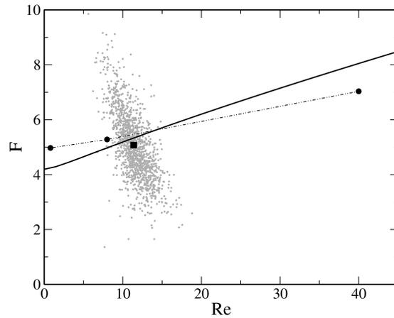
FIGURE 5. Dimensionless drag force as function of the particle Reynolds number with an overall gas volume fraction of 0.8. Comparison between the Beetstra *et al.* (2007) model (line), a stationary random arrangements of spheres (filled circles, dashed line), and moving spheres (average value (square) and scatter plot of forces on individual particles (grey dots) obtained using a filter size  $\Delta = 15d_p$ .)
