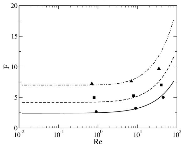
FIGURE 4. Non-dimensional drag force as function of the particle Reynolds number for random arrangements of spheres. Comparison between the model of Beetstra *et al.* (2007) (lines) and present work (symbols).  $\varepsilon = 0.9$  (circles),  $0.8$  (squares), and  $0.7$  (triangles).
