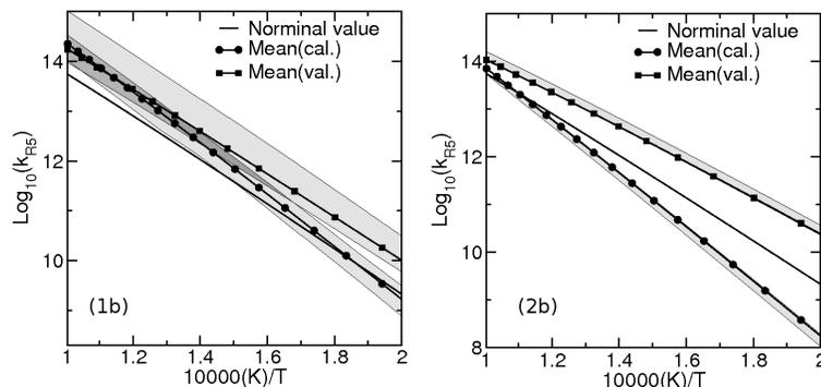
FIGURE 4. Posterior mean and 95% confidence interval (CI) for the log reaction rates ( $k_{R5}$ ) versus  $10^4(K)/T$ . Results from the one-temperature model and from the two-temperature model are shown on the left plot and on the right plot, respectively. The gray region represents the 95% confidence interval.
