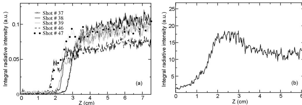
FIGURE 3. Spectrally integrated radiance versus distance along the shock-tube access. The spectral integration interval is 772–782 [nm]. (a) calibration data and (b) validation data (from Cruden *et al.* (2009)).
