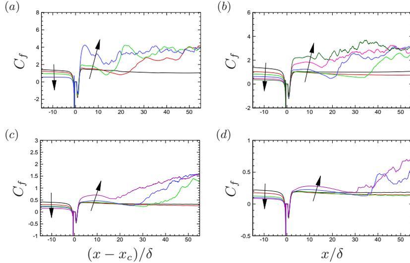
FIGURE 1. Mean skin friction coefficient along the symmetry line for hemispherical roughness element with size  $k/\delta = 0.4$ . (a),  $M_\infty = 1.1$ ,  $Re_\delta = 2500, 2900, 3655, 6500$ ; (b),  $M_\infty = 2$ ,  $Re_\delta = 3000, 4000, 5000, 65000, 9000, 11500$ ; (c),  $M_\infty = 4$ ,  $Re_\delta = 15000, 20000, 25000, 28000, 40000$ ; and (d),  $M_\infty = 6$ ,  $Re_\delta = 40000, 50000, 70000, 85000, 100000$ . The arrows indicate the direction of increasing  $Re_\delta$ .
