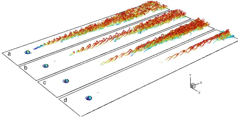
FIGURE 2. Coherent vortical structures for flow around hemispherical roughness element. (a),  $M_\infty = 1.1$ ,  $Re_\delta = 6500$ ; (b),  $M_\infty = 2$ ,  $Re_\delta = 9000$ ; (c),  $M_\infty = 4$ ,  $Re_\delta = 40000$ ; and (d),  $M_\infty = 6$ ,  $Re_\delta = 85000$ . Vortices are educed as isosurfaces of swirling strength, and colored with the streamwise velocity.
