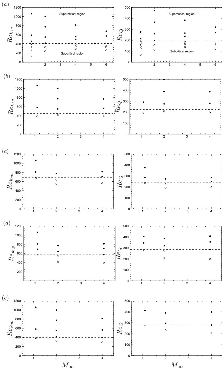
FIGURE 5. Transition map as a function of  $Re_{kw}$  (left column) and  $Re_Q$  (right column). (a) hemispheres; (b) cubes; (c) cylinders ( $D/k = 1/2$ ); (d) cylinders ( $D/k = 1$ ); (e) cylinders ( $D/k = 2$ ). Solid/open circles denote super/sub critical cases.
