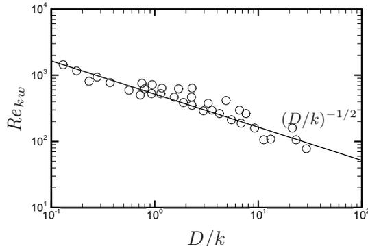
FIGURE 6. Dependence of critical roughness Reynolds number on obstacle aspect ratio (*solid line*, Eq. (5.5); *symbols*, experimental data (Schneider 2008))
