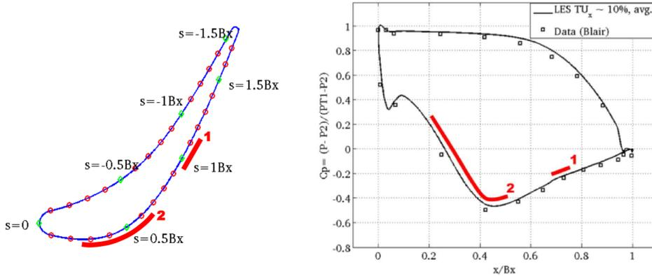
FIGURE 1. Definition of curvilinear coordinate  $s$  (left) where  $B_x$  is the axial chord of the airfoil, and plot of pressure coefficient  $C_P = (P - P_2)/(P_{T1} - P_2)$  vs axial coordinate  $x$ , computed on baseline grid (right). Stripes 1 and 2 indicate where transition takes place in the experiment — without and with the presence of turbulence grid.
