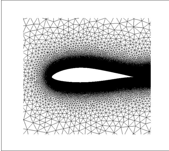
FIGURE 1. Hybrid grid generated around the DU96 airfoil. Note that the grid is structured in the near field and unstructured in the far field.
