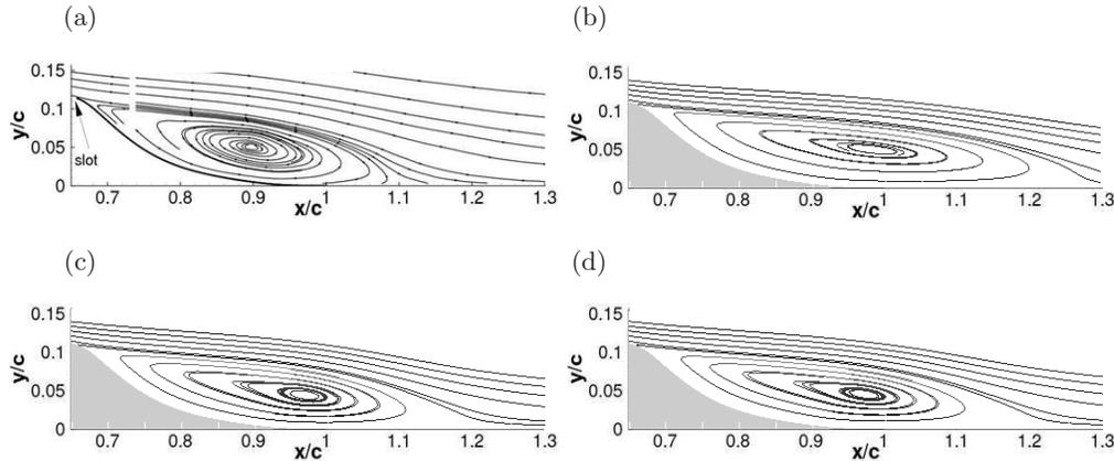
FIGURE 3. Comparison of velocity streamlines for (a) experimental results (Viken *et al.* 2003) and simulations using (b) a wall-resolved grid, (c) analytic wall functions and (d) tabulated wall functions.
