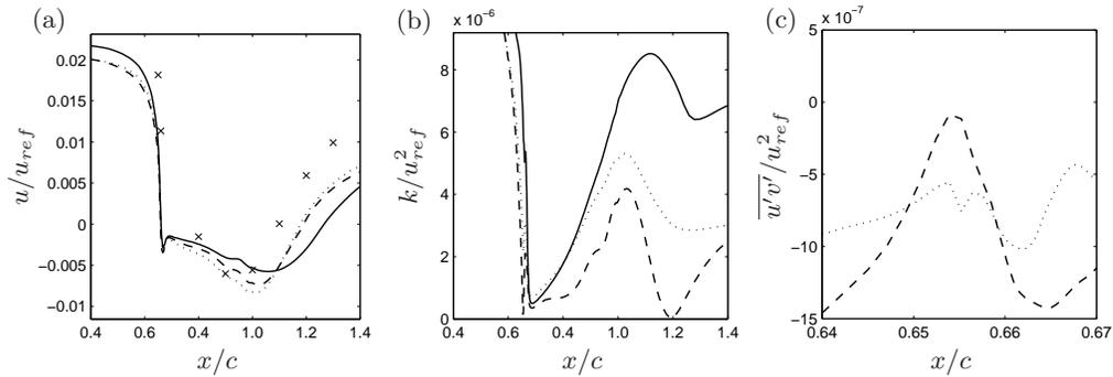
FIGURE 4. Plots comparing (a) streamwise velocity (b) turbulent kinetic energy and (c) Reynolds shear stress obtained at constant wall-normal distance for simulations using a wall-resolved grid (—), analytic wall functions (...) and tabulated wall functions(- -). Experimental results (Viken *et al.* 2003) also shown ( $\times$ ).
