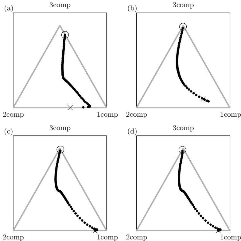
FIGURE 1. Barycentric maps for the trajectory from the center of the duct to the center of the bottom wall comparing (a) DNS results (b) no wall blocking (c) scalar wall blocking and (d) vector wall blocking. Start of the trajectory indicated with (o) and the end with (x).
