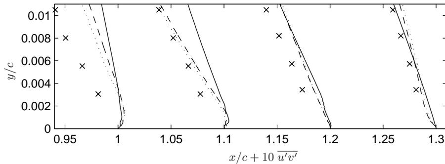
FIGURE 5. Plot comparing Reynolds shear stress for simulations using a wall-resolved grid (—), analytic wall functions (...) and tabulated wall functions(- -). Experimental results (Viken *et al.* 2003) also shown ( $\times$ ).
