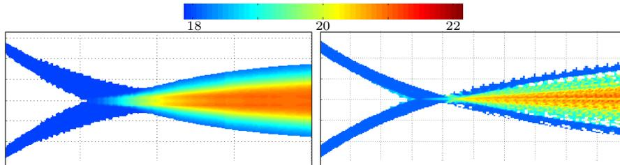
FIGURE 6. Volume average radius  $r_{30}$  ( $\mu\text{m}$ ) of the overall distribution – Left: Eulerian (SAP2); Right: Time average Lagrangian (Asphodele).
