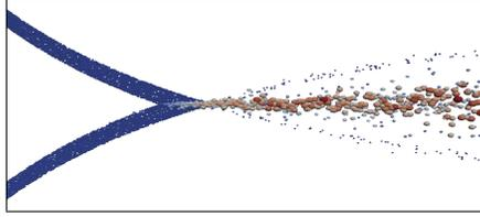
FIGURE 3. Instantaneous location of particles colored by size for  $\text{Kn}_{\text{coal}} = 1$  with Lagrangian approach (Asphodele).
