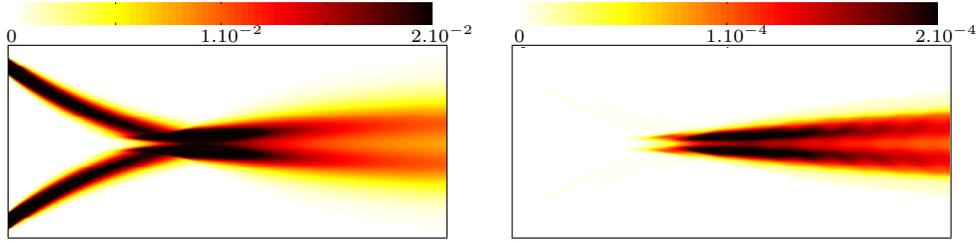
FIGURE 2. Mass concentration ( $\text{kg}/\text{m}^3$ ) for  $\text{Kn}_{\text{coal}} = 100$  with Eulerian approach (SAP2) – Left: Section 1 (mode 0); Right: Section 2 (mode 1).
