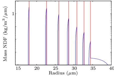
FIGURE 4. Mass density function (log-scale) at the output on centerline for  $\text{Kn}_{\text{coal}} = 1$  with Eulerian approach (SAP2).
