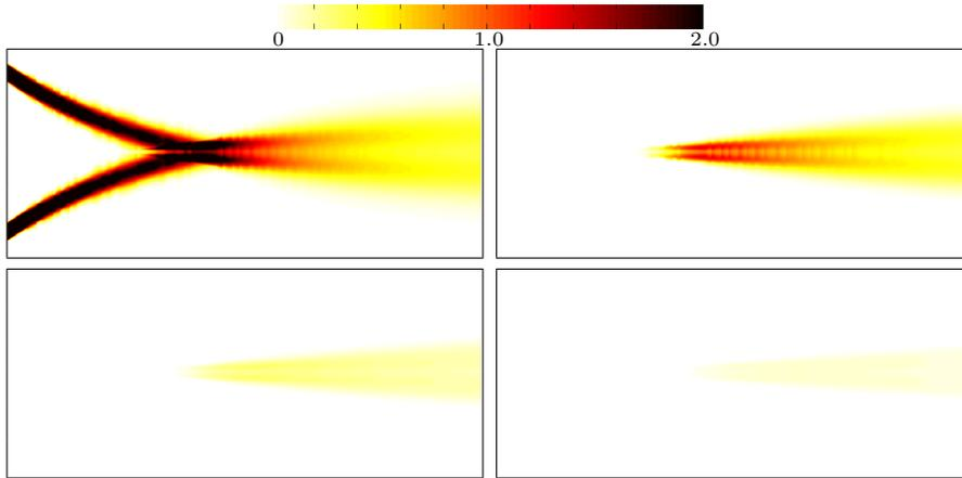
FIGURE 5. Mass concentration per section with Eulerian approach (SAP2) – Top left to bottom right: section 1 to 4
