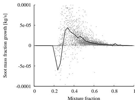
FIGURE 5. Soot mass fraction growth at time  $t = 20$  ms; results shown for SIM-A. Every point represents a Lagrangian particle and the time derivative is computed on the Lagrangian trajectory. Only a small fraction of the entire set of particles is shown. Mean soot mass fraction growth conditioned on mixture fraction (line).
