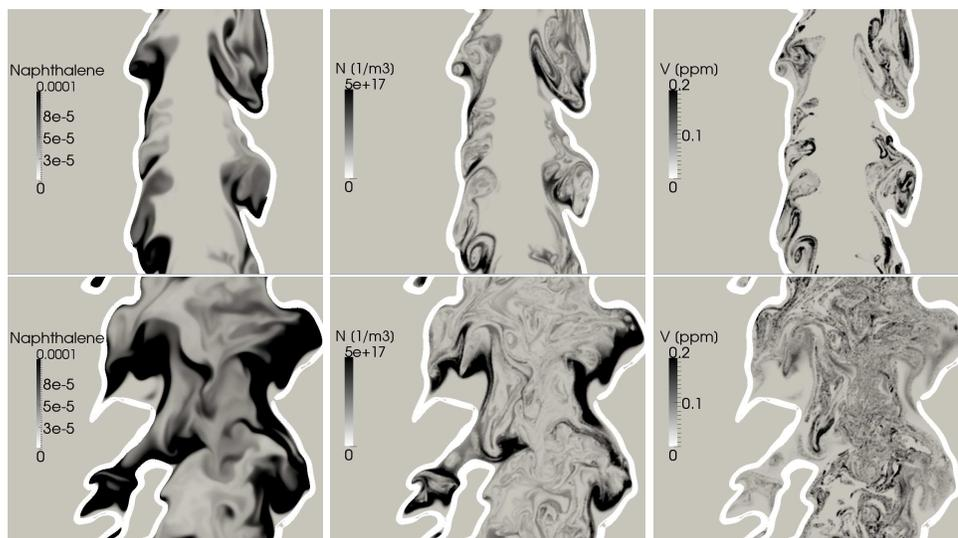
FIGURE 1. Naphthalene (left), soot number density (center), and soot volume fraction (right) at 10 ms (top) and 25 ms (bottom) for SIM-A. The flame is highlighted by the white lines, representing high concentration of HCO.
