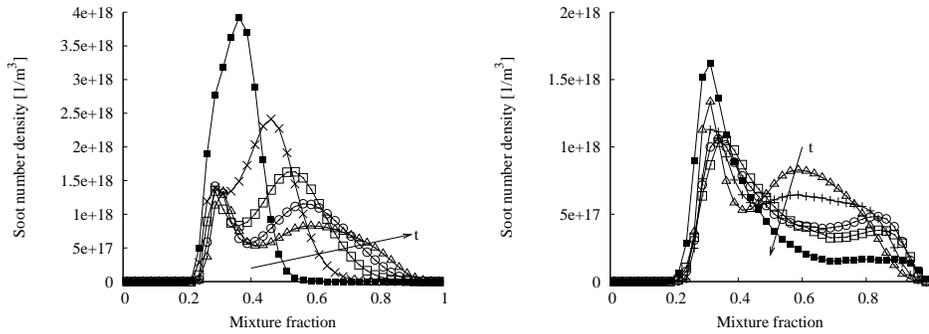
FIGURE 2. Mean number density of soot particulate, conditioned on mixture fraction, at several time instants; results shown for SIM-A. Left figure: number density at 1 ms (filled squares), 2 ms (crosses), 3 ms (open squares), 4 ms (circles), and 5 ms (triangles). Right figure: number density at 5 ms (triangles), 6 ms (plus), 8 ms (circles), 10 ms (open squares), and the late time solution at 25 ms (filled squares). The scale of the number density axes is different in the two figures.
