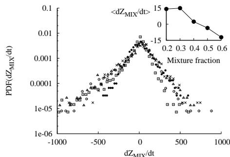
FIGURE 6. PDFs of Lagrangian time derivative of mixture fraction conditioned on several values of mixture fraction at time  $t = 20$  ms; results shown for SIM-A.  $Z = 0.2$  (filled circles),  $0.3$  (crosses),  $0.4$  (open triangles),  $0.5$  (open circles),  $0.6$  (open squares). Inset: mean value for the distributions shown in the main figure.
