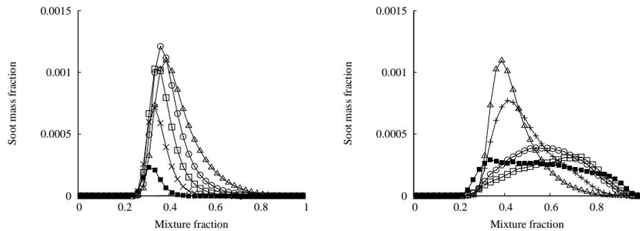
FIGURE 4. Mean mass fraction of soot particulate, conditioned on mixture fraction, at several time instants; results shown for SIM-A. Left figure: mass fraction at 1 ms (filled squares), 2 ms (crosses), 3 ms (open squares), 4 ms (circles), and 5 ms (triangles). Right figure: mass fraction at 5 ms (triangles), 6 ms (plus), 8 ms (circles), 10 ms (open squares), and the late time solution at 25 ms (filled squares).
