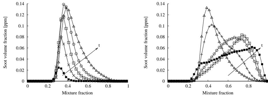
FIGURE 3. Mean volume fraction of soot particulate, conditioned on mixture fraction, at several time instants; results shown for SIM-A. Left figure: volume fraction at 1 ms (filled squares), 2 ms (crosses), 3 ms (open squares), 4 ms (circles), and 5 ms (triangles). Right figure: volume at 5 ms (triangles), 6 ms (plus), 8 ms (circles), 10 ms (open squares), and the late time solution at 25 ms (filled squares).
