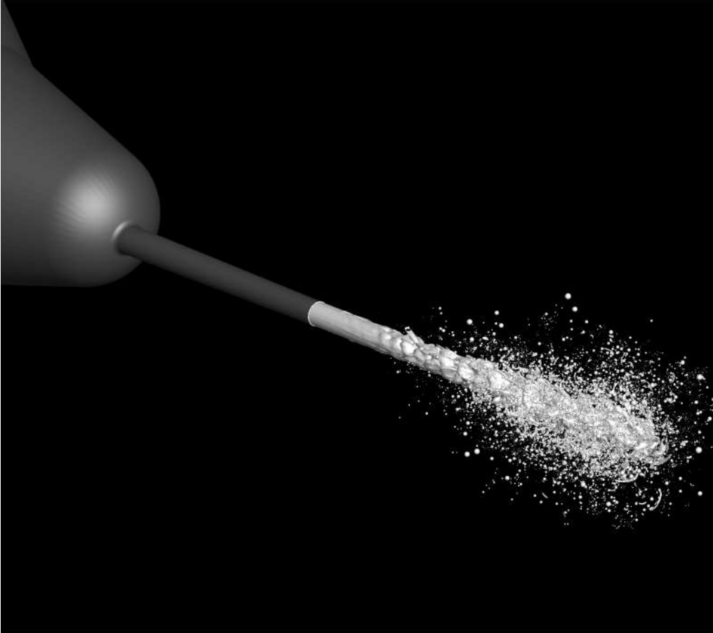
FIGURE 7. Volume fraction isosurface and Lagrangian particles alongside the diesel spray injector.
