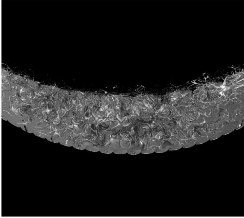
FIGURE 5. Q criterion isosurface shaded by streamwise velocity at the bottom wall of the diesel spray injector as viewed from downstream.
