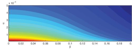
FIGURE 5: Transfer function linking coherent streamwise-velocity structures and coherent streamwise-velocity autocorrelation, visualized by contours in the streamwise-spanwise wavenumber plane.
