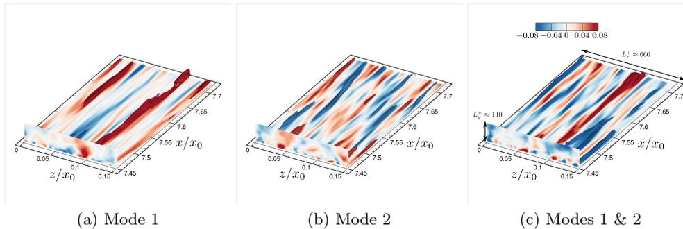
FIGURE 4: Coherent structures of low frequency, visualized by the streamwise velocity component. Streamwise and spanwise directions are normalized by  $x_0$ , where  $Re|_{x_0} = 10^5$ .
