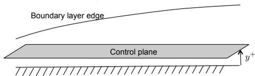
FIGURE 1: Schematic of the location of the sensing-and-control plane.
