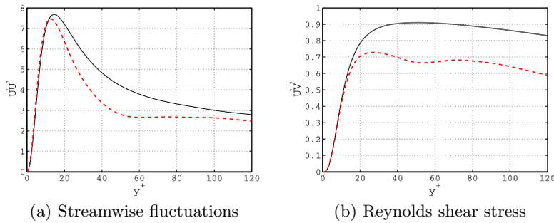
FIGURE 3: The contribution of the coherent structures to the fluctuating shear stresses. —, total shear stress; - - -, contribution from mode 4 and mode 6.
