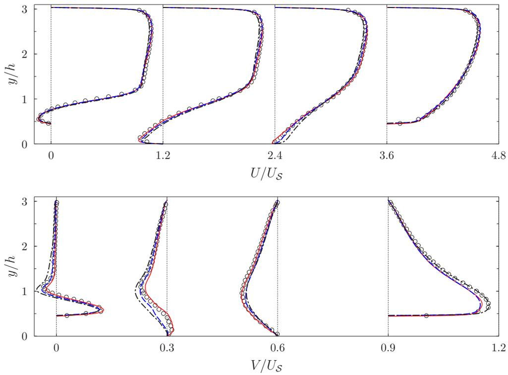
FIGURE 2. Mean velocity profiles in the streamwise ( $U$ ) and vertical ( $V$ ) directions (color online). From left to right, velocity profiles at  $x/h = 1, 2, 4$ , and  $8$ . Red solid lines, DNS (case 1); blue dashed lines, LES (case 2); black dash-dotted lines, ILES (case 3); circles, experiment (Breuer *et al.* 2009).
