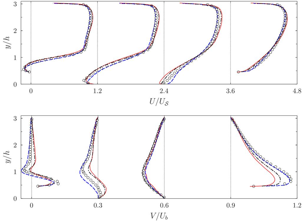
FIGURE 5. Mean velocity profiles in the streamwise ( $U$ ) and vertical ( $V$ ) directions (color online). From left to right, velocity profiles at  $x/h = 1, 2, 4$ , and  $8$ . Red solid lines, slip WM (case 4); blue dashed lines, non-equilibrium WM (case 5); black dash-dotted lines, equilibrium WM (case 6); circles, experiment (Breuer *et al.* 2009).
