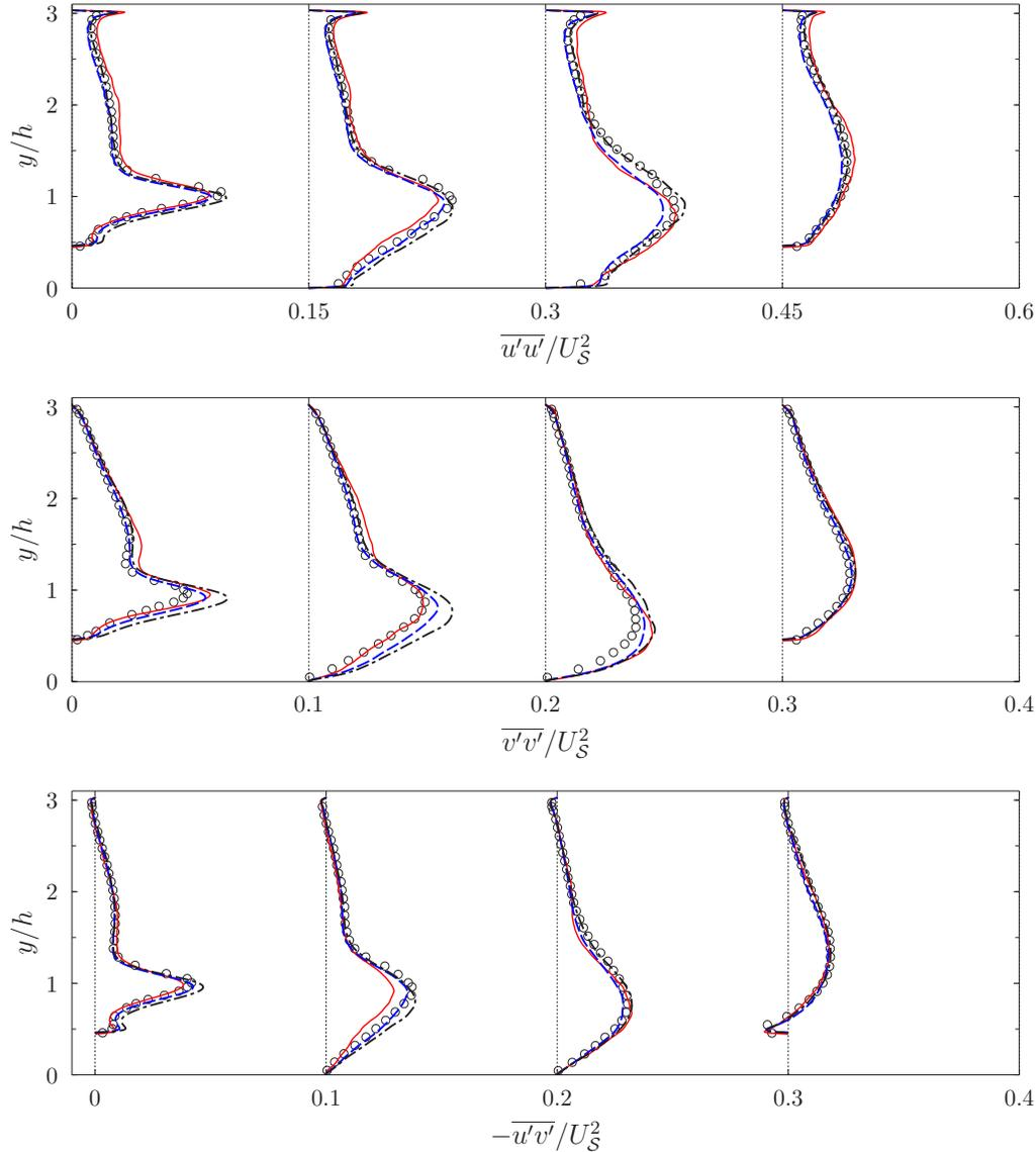
FIGURE 4. Profiles of Reynolds stresses at  $x/h = 1, 2, 4,$  and  $8$  (from left to right, color online). Red solid lines, DNS (case 1); blue dashed lines, LES (case 2); black dash-dotted lines, ILES (case 3); circles, experiment (Breuer *et al.* 2009).
