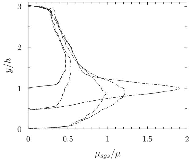
FIGURE 3. Variation of the SGS eddy viscosity at different stations (case 2). Solid line,  $x/h = 0$ ; dashed line,  $x/h = 1$ ; dash-dotted line,  $x/h = 2$ ; dash-dot-dot-dotted line,  $x/h = 4$ ; dash-dot-dotted line,  $x/h = 8$ .
