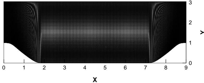
FIGURE 1. Side view of the mesh used for LES and WMLES calculations.
