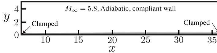
FIGURE 4. Spatial domain used in global stability solution. The inflow and outflow values of  $R$  are 1000 and 1700, respectively, and correspond to locations of clamped-clamped boundary conditions.
