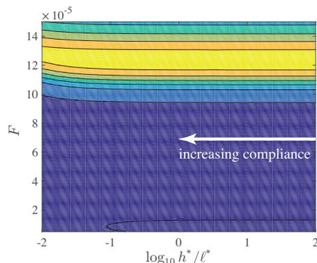
FIGURE 2. Contours of  $-\alpha_i^* \delta_0^*$  as a function of panel thickness  $h^*$  for a Mach 5.8 boundary layer at  $R = 1000$ ,  $\beta = 0$  for Hastelloy-X. Contour levels are logarithmically spaced between  $[10^{-5}, 10^{-1}]$ .
