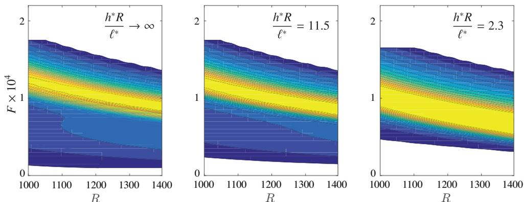
FIGURE 3. Contours of  $-\alpha_i^* \delta_0^*$  as functions of  $F$  and  $R$  for a Mach 5.8 boundary layer with  $\beta = 0$  for Hastelloy-X. Contour levels are logarithmically spaced between  $[10^{-5}, 10^{-1}]$ .
