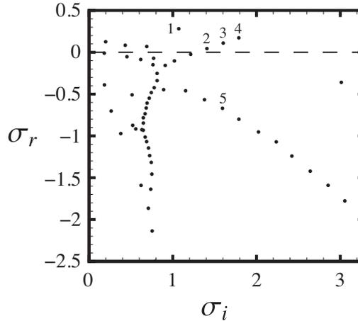
FIGURE 5. Discrete spectrum of the FTSI-coupled global stability solver for the case described in figure 4. Identified modes are shown in figure 6.
