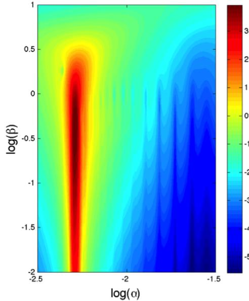
FIGURE 4: Wavenumber-corrected norm of the transfer function describing the mapping of the coherent normal velocity  $\hat{v}$  to the coherent stress component  $\hat{r}_{uu}$  in the wall-parallel input-output plane at  $y^+ = 25$ . The transfer function has been evaluated for  $\omega = 0.066$ , the dominant frequency extracted by DMD from the numerical simulation. The contours are plotted logarithmically.
