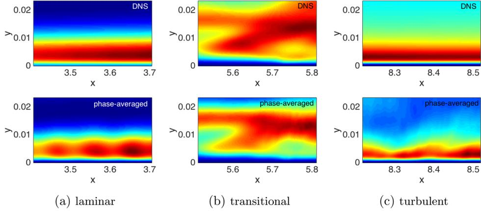
FIGURE 3: Comparison of the phase-averaged and the total streamwise fluctuation data in three different regimes of laminar, transitional and turbulent flow, as highlighted in the boxed areas of Figure 2(a).
