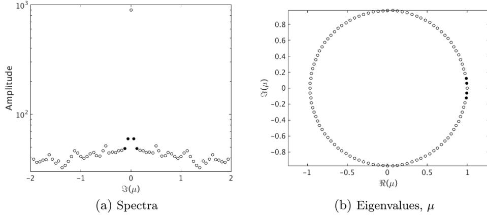
FIGURE 1: Eigenvalue and spectra of the DMD modes for the whole-domain analysis. The two low-frequency modes are highlighted using filled symbols.
