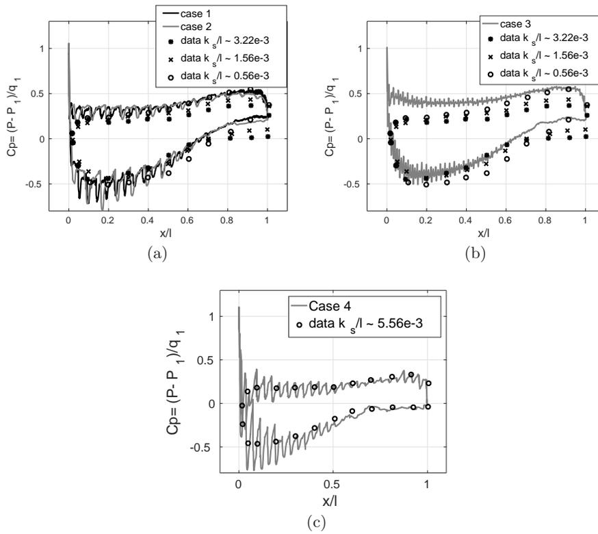
FIGURE 7. Spanwise averaged blade loadings; (a) case 1 and 2; (b) case 3; (c) case 4.
