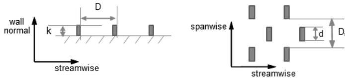
FIGURE 2. Schematic of discrete roughness element configuration.
