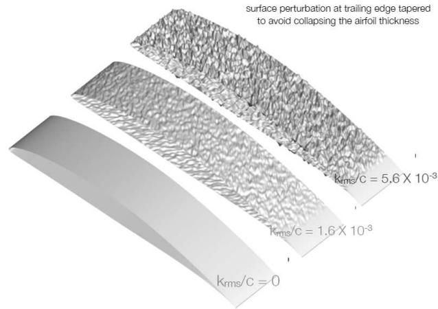
FIGURE 4. Geometry of randomly distributed roughness for unstructured solver
