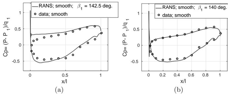
FIGURE 5. Blade loading of smooth blade; (a) default inflow angle,  $\beta_1 = 142.5^\circ$ , (b) adjusted inflow flow angle,  $\beta_1 = 140^\circ$ .
