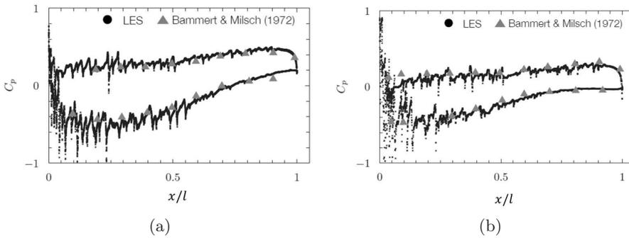
FIGURE 8. Blade loadings of randomly distributed roughness cases; (a)  $k_{rms}/l \sim 1.56 \times 10^{-3}$ ; (b)  $k_{rms}/l \sim 5.56 \times 10^{-3}$ .
