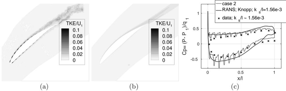
FIGURE 9. (a), (b) contours of turbulence kinetic energy normalized by flow velocity at inflow of case 2 and RANS with Knopp roughness model with  $k_s/l = 1.56 \times 10^{-3}$ ; (c) blade loadings
