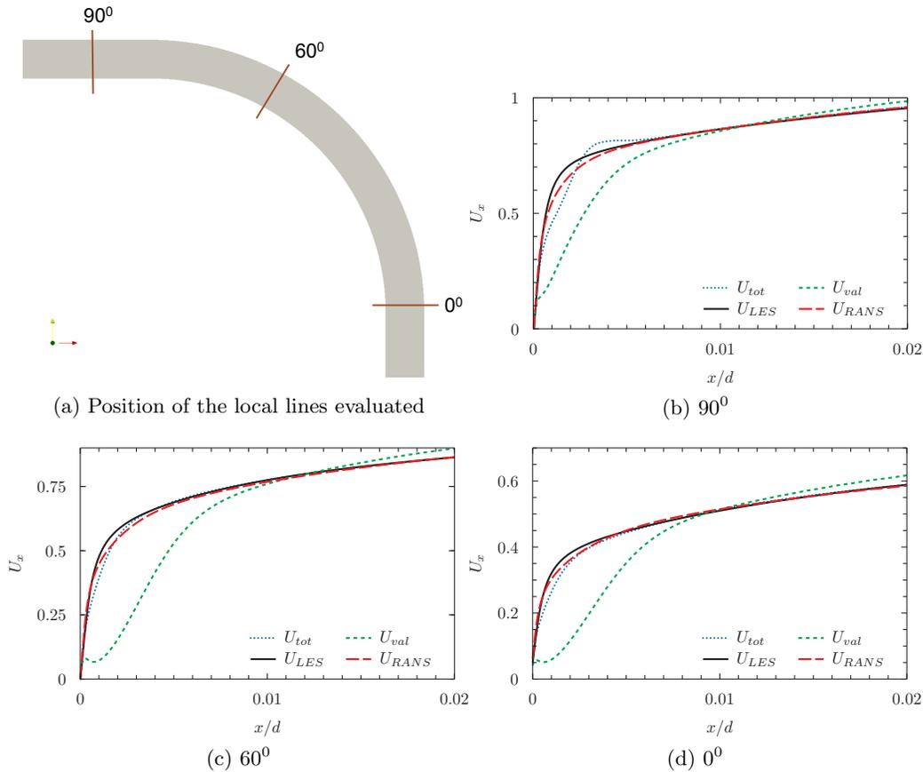
FIGURE 5. Velocity profiles corresponding to four cases: LES, RANS, RANS with perturbed eigenvalues ( $U_{val}$ ), RANS with perturbed eigenvalues and eigenvectors ( $U_{tot}$ )
