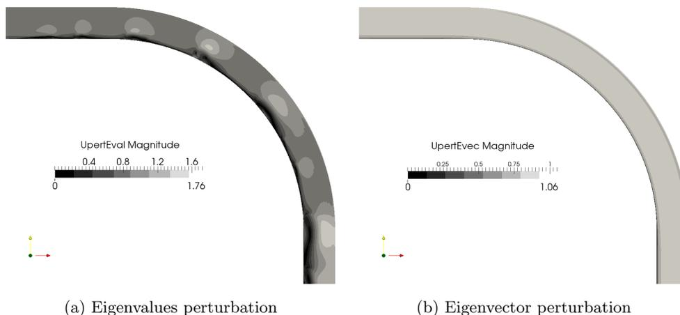
FIGURE 4. Magnitude difference between the perturbed RANS velocity and LES velocity.
