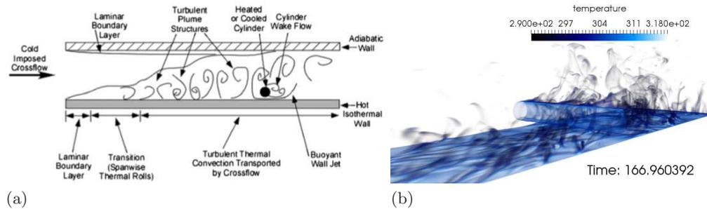
FIGURE 1. (a) Details of the experimental configuration — figure reproduced from Kearney *et al.* (2005). (b) Representative volume-rendered temperature field from LES simulation with thermal plumes depicted.
