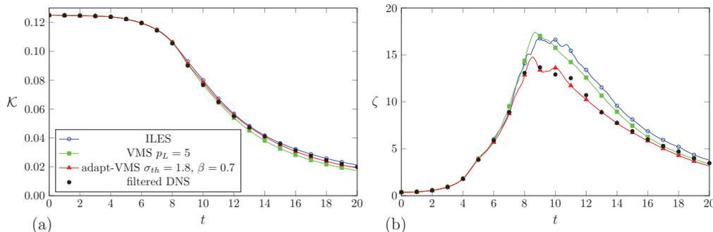
FIGURE 4. TGV at  $Re = 5,000$ : evolution of the (a) resolved kinetic energy and (b) enstrophy.
