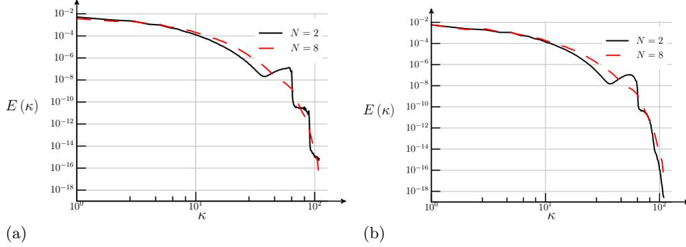
FIGURE 3. Computed energy spectrum for HIT using 128 dof at  $Ma_t = 0.1$ ,  $Re_\lambda = 45$ . (a) Entropy conservative; (b) entropy stable.
