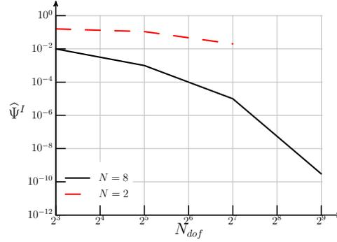
FIGURE 4. Convergence of the inviscid entropy stabilization term,  $\widehat{\Psi}^I$ , with increasing resolution.  $Ma_t = 0.1$ ,  $Re_\lambda = 45$ .
