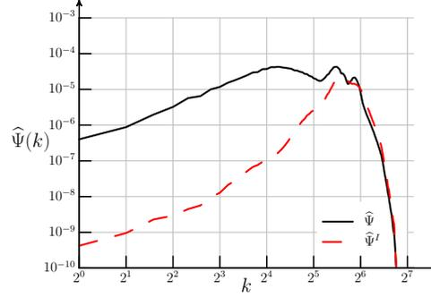
FIGURE 5. Computed energy spectrum for the entropy production terms for the HIT using 128 dof at  $Ma_t = 0.1$  and  $Re_\lambda = 45$ .
