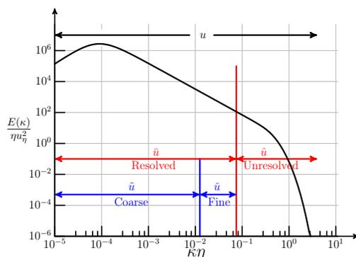
FIGURE 1. *A priori* scale separation for a variational multiscale method following the triple decomposition of Collis (2001).
