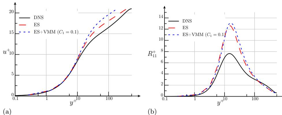
FIGURE 2. Computed velocity profiles and Reynolds stress for channel flow at  $Re_\tau = 544$ . (a) Mean velocity; (b)  $R_{11}$  Reynolds stress. DNS data from Lee & Moser (2015).
