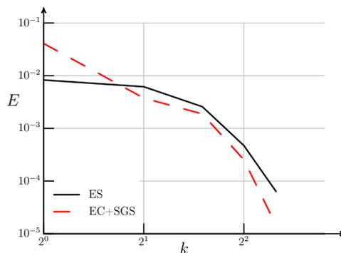
FIGURE 6. Computed energy spectrum for HIT using 8 dof at  $Ma_t = 0.1$ ,  $Re_\lambda = 45$ .
