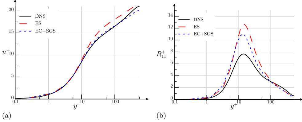
FIGURE 8. Computed velocity profiles and Reynolds stress for channel flow at  $Re_\tau = 544$ . (a) Mean velocity; (b)  $R_{11}$  Reynolds stress. DNS data from Lee & Moser (2015).
