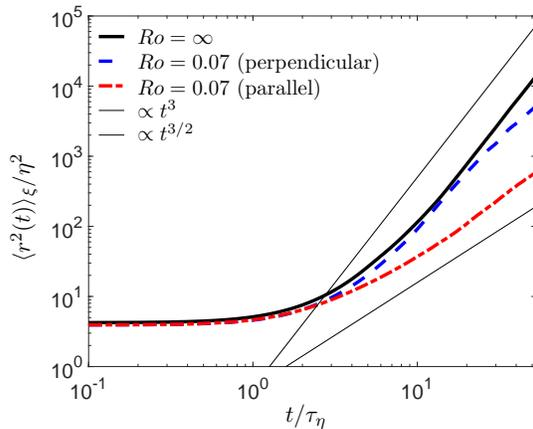
FIGURE 1. DNS results for  $\langle r^2(t) \rangle_\xi$  for fluid particles with initial separation  $\xi \in [1, 2]\eta$ . The black solid line corresponds to the simulation without rotation,  $Ro = \infty$ , for which the dispersion is isotropic, and the blue dashed and red dashed-dot lines correspond to dispersion in the directions perpendicular and parallel to the rotation axis, respectively, for a flow with  $Ro = 0.07$ .
