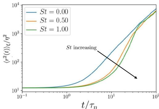
FIGURE 3. DNS results for  $\langle r^2(t) \rangle_\xi$  for particles with different  $St$ . In this simulation, the fluid flow is subject to rotation with  $Ro = 0.07$ , however, in the particle equation of motion the Coriolis and centrifugal terms are switched off in order to investigate the implicit effects of rotation.
