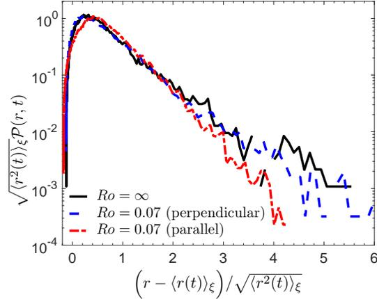
FIGURE 2. DNS results for  $\mathcal{P}(r, t)$  for fluid particles with initial separation  $\xi \in [1, 2]\eta$ , plotted in standard form. The black solid line corresponds to the simulation without rotation  $Ro = \infty$ , for which the dispersion is isotropic, and the blue dashed and red dashed-dot lines correspond to dispersion in the directions perpendicular and parallel to the rotation axis, respectively, for a flow with  $Ro = 0.07$ .
