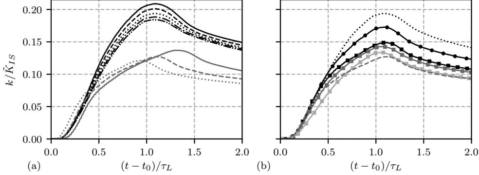
FIGURE 4. Mean fluctuating kinetic energy over  $x/L = 0.1$  to  $x/L = 0.9$ . Solid black line: case I, black dashed line: case II, black dotted line: case III, black dash-dotted line: case IV, black dashed and double-dotted line: case V, black line and circles: case VI, black squares: case VII, dark grey squares: case VIII, light grey squares: case IX, grey solid line: case X, grey dashed line: case XI, grey dotted line: case XII.
