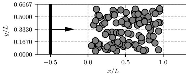
FIGURE 1. Sketch of the 3D simulation problem setup. A shock wave, shown in the left part of the figure passes through the cloud of particles located between  $x/L = 0$  and  $x/L = 1$ .
