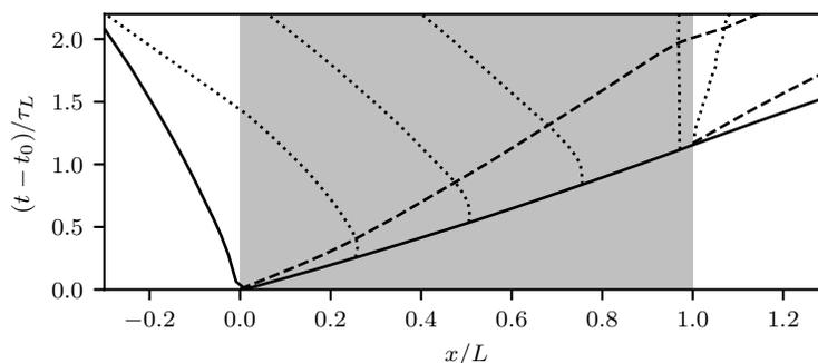
FIGURE 2. Wave diagram showing the positions of the incident, transmitted and reflected shock waves (solid lines), upstream and downstream contacts (dashed lines) and acoustic waves (dotted lines) in case VII. The particle cloud is indicated by the grey region.
