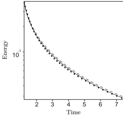
FIGURE 1. Decay of the resolved energy for truncated DNS ( $\bullet$ ), LES with the dynamic Smagorinsky model (-----) and LES with the dynamic Smagorinsky model and the  $\tau$  term (—).
