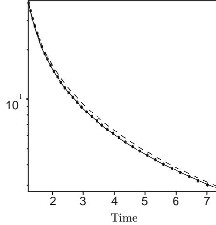
FIGURE 2. Decay of the resolved energy for truncated DNS ( $\bullet$ ), LES with the dynamic Kolmogorov model (-----) and LES with the dynamic Kolmogorov model and the  $\tau$  term (—).
