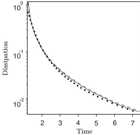
FIGURE 3. Decay of the resolved dissipation for truncated DNS ( $\bullet$ ), LES with the dynamic Smagorinsky model (-----) and LES with the dynamic Smagorinsky model and the  $\tau$  term (—).
