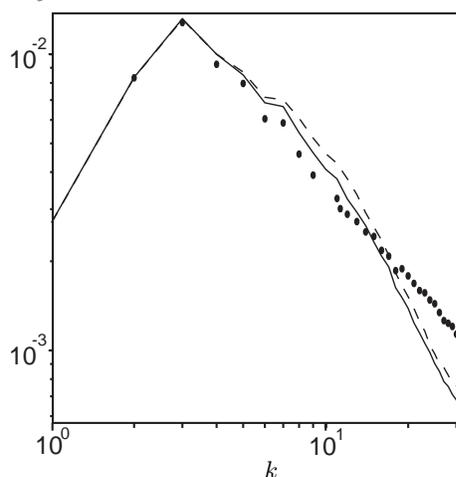
FIGURE 6. Energy spectrum at  $t = 2.6$  in the units of Figs. 1-4 for truncated DNS ( $\bullet$ ), LES with the dynamic Kolmogorov model (-----) and LES with the dynamic Kolmogorov model and the  $\tau$  term (—).
