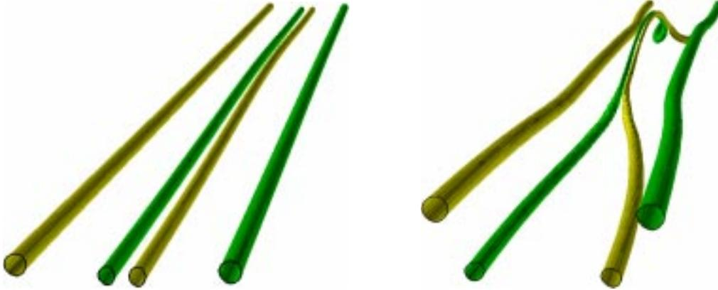
FIGURE 3. Initial stage (left) and reconnection for a configuration of two vortex pairs of opposite sign, according to Rennich & Lele (1998). Courtesy of S. Lele.
