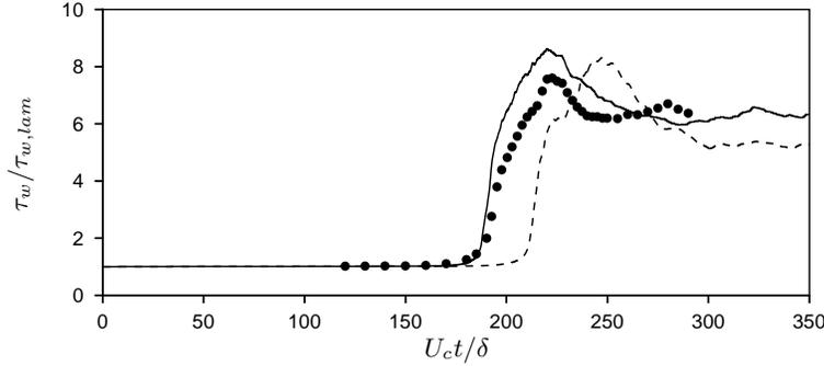
FIGURE 2. Time history of average wall shear stress from the transitional channel simulation. — fine LES ( $32 \times 128 \times 64$ ); - - - coarse LES ( $32 \times 64 \times 32$ ); • DNS of Zang *et al.* (1990)
