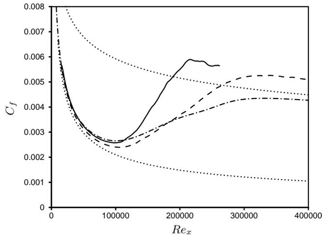
FIGURE 5. Comparison of time averaged skin friction coefficient along flat plate, — LES; - - - RANS; - - - DNS of Wu *et al.* (1999); ..... laminar and turbulent correlations.
