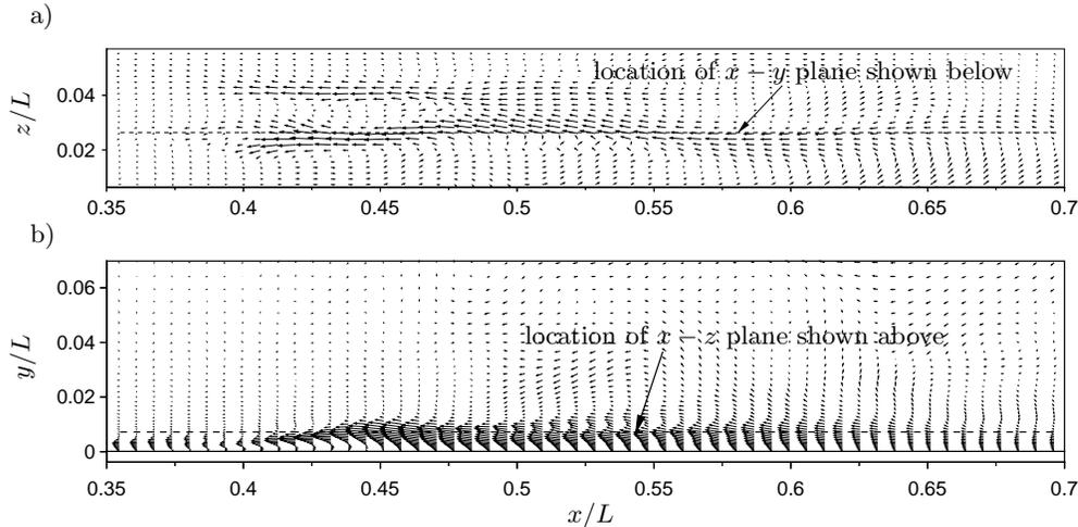
FIGURE 4. Fluctuating velocity vectors upstream of a future turbulent spot showing backward jet structure. a)  $x-z$  plane; b)  $x-y$  plane.
