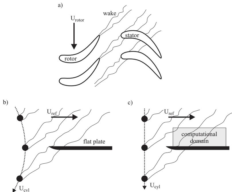
FIGURE 1. a) Schematic of rotor-stator wake interaction; b) layout in the experiments of Liu and Rodi (1991); c) layout in the DNS of Wu *et al.* (1999), and the present LES and RANS.
