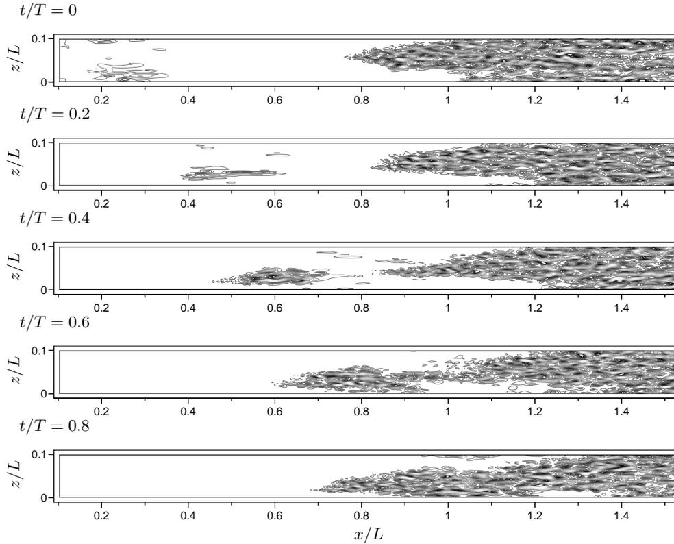
FIGURE 3. Visualization of turbulent spot formation and growth using v-component of fluctuating velocity in the x-z plane near the wall ( $y/\delta_{99} = 0.4$  at  $x/L = 0.8$ ). Contours represent  $-0.1 < v/U_{ref} < 0.1$  in 0.01 increments.
