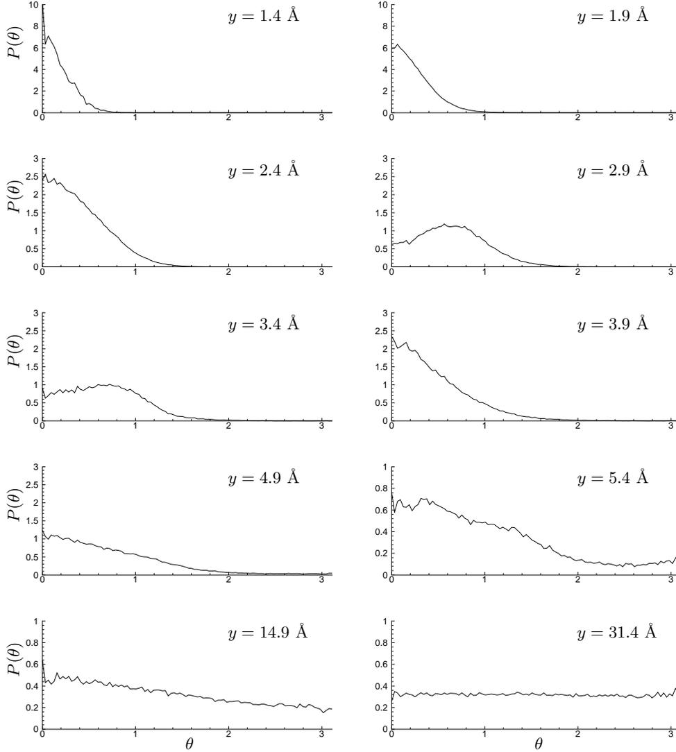
FIGURE 5. Probability density function of water molecule orientations. The angle  $\theta$  is defined in figure 4. The  $y$ -locations correspond to the center of the oxygen atom.
