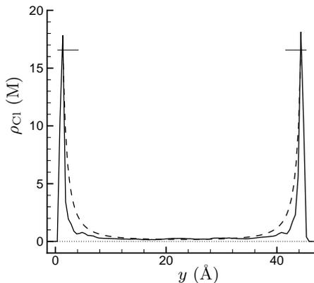
FIGURE 3. Chloride number density: — simulation; ---- (1.1) with  $\psi$  from (1.3). The ..... line is  $\rho_{\text{Cl}} = 0$ . The horizontal line segments demark the peak reached by the ---- curve.
