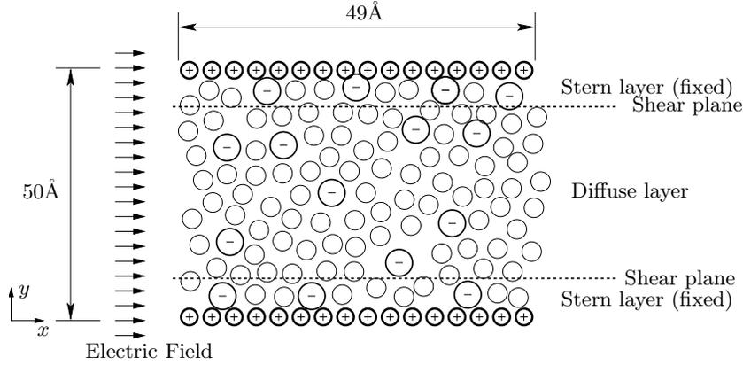
FIGURE 1. Schematic of the electric double layer in a nanometer-scale channel. For simplicity both this schematic and the present simulations only have counter ions in the solution. Two dimensions of the simulated channel are labeled. It also extends  $49\text{\AA}$  in the  $z$ -direction.
