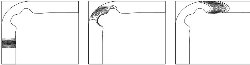
FIGURE 8. Second class of optimized shapes for the 90-degree turn. The magnitude of the skew is about the same than for the first class above with 15% less reduction in cross-section, but there is more dispersion in the advection band as the wall curvature variation is higher.
