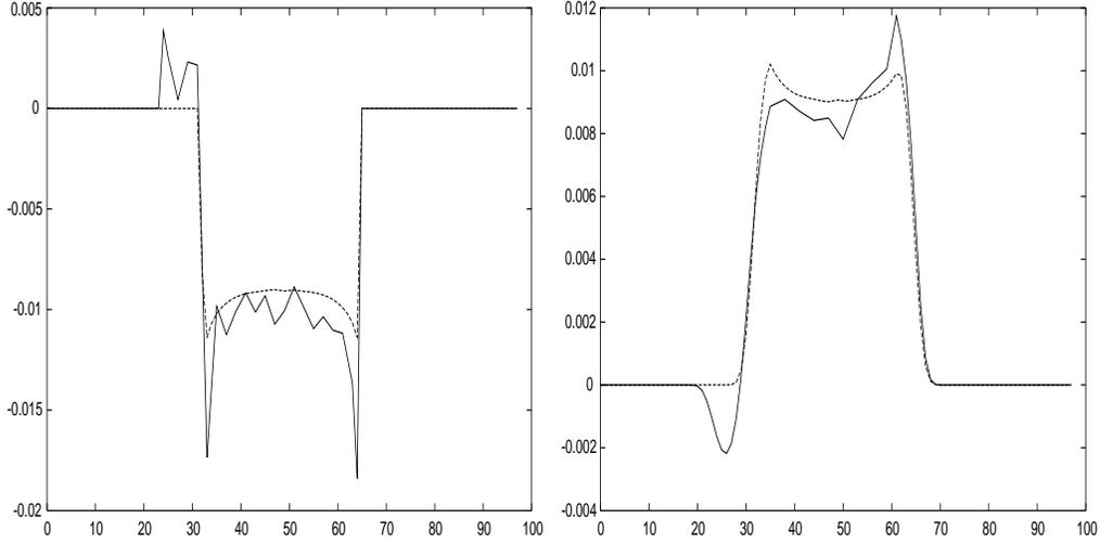
FIGURE 2. Sensitivity evaluation around the initial 90-degree turn for control points along the inner channel wall. Comparison between the exact (—) and incomplete (---) gradient evaluations (left). The deformations obtained using these gradients (right).
