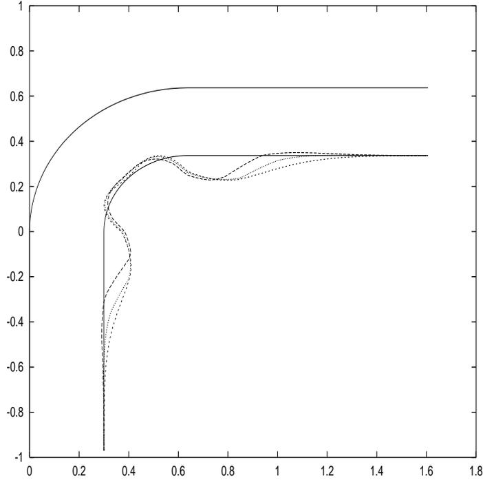
FIGURE 1. Shapes obtained under the same optimization conditions for three admissible spaces with different minimum required regularity for the shape. I: initial (—), II: less regular (---), III: medium regularity (-.-.-), IV: most regular (.....).
