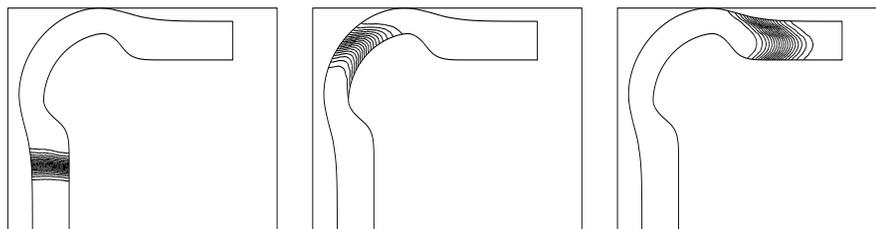
FIGURE 10. Third class of optimized shapes for the 90-degree turn with both the inner and outer walls modified. The skew is about the same than for the first class of the 90-degree optimized turn but with a much larger cross-section, but also more band dispersion away from walls.
