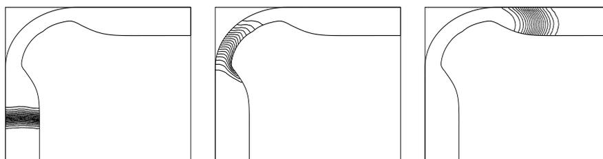
FIGURE 6. First class of optimized shapes for the 90-degree turn. The magnitude of the skew has been reduced by one order.
