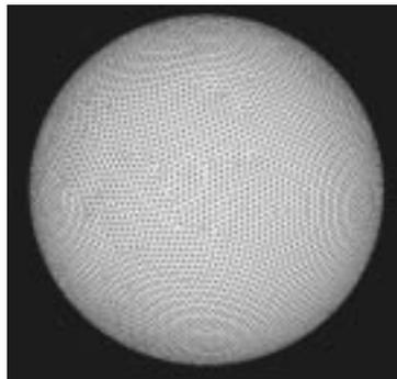
FIGURE 2. Finite element mesh on the truncating surface.
