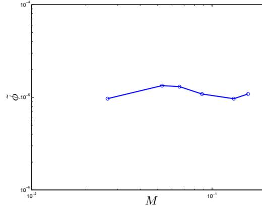
FIGURE 10. Total far-field acoustic intensity  $\tilde{\phi}$  as a function of Mach number  $M$ , for  $\omega = 10.14$ .
