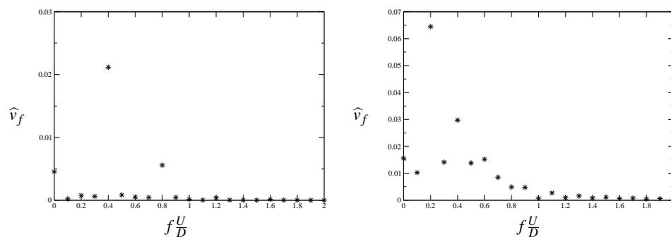
FIGURE 11. Spectra of the vertical velocity of the flow at  $\{x,y\} = \{1.5D, 0.5D\}$  (left) and  $\{x,y\} = \{3D, 0.5D\}$  (right). The appearance of the peak at  $S_t = 0.2$  at the downstream station (right) is a result of vortex pairing (recall that the jet is forced at  $S_t = 0.4$ ).
