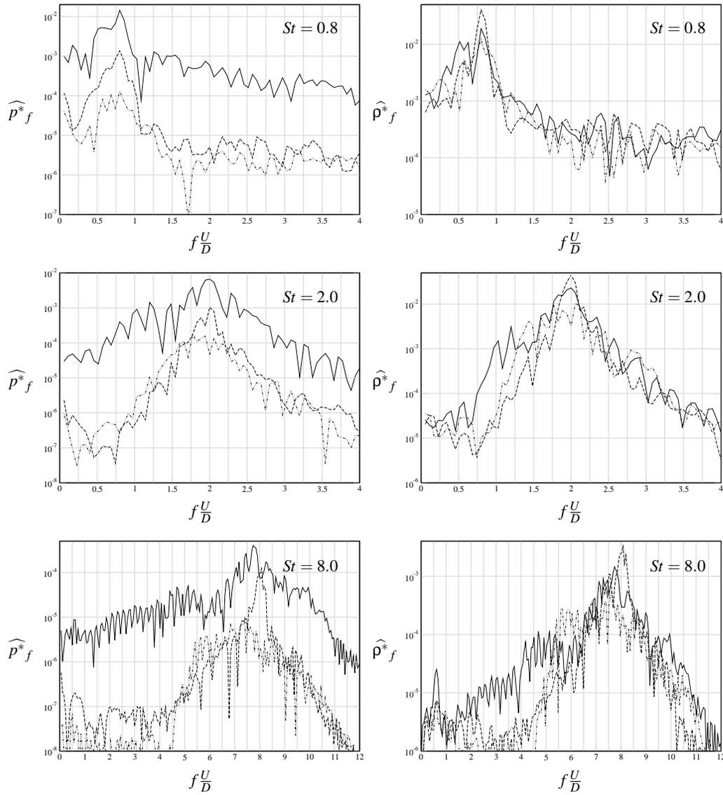
FIGURE 10. Temporal spectra of (left) the adjoint pressure  $\widehat{p}^*_f$  and (right) the adjoint density  $\widehat{\rho}^*_f$  for an incident wave in the adjoint field coming from above (at an angle of  $60^\circ$  off the jet axis), at a frequency of (top)  $St = 0.8$ , (middle)  $St = 2.0$ , and (bottom)  $St = 8.0$  and measured at the points  $\{x, y\}$  of (solid)  $\{5D, 0\}$ , (dashed)  $\{5D, 2.5D\}$ , (dot-dashed)  $\{5D, -2.5D\}$ . See Figure 9 for flow configuration.
