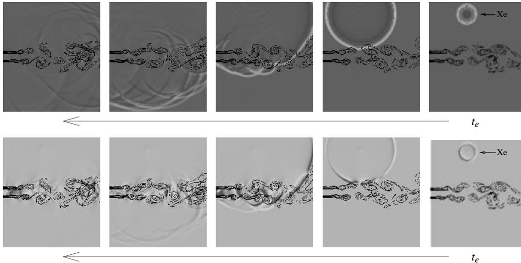
FIGURE 5. Adjoint density (top) and adjoint pressure (bottom) reveals sensitivity of the pressure component of the perturbation field at point  $x_e$  at time  $t_e$  to additional forcing of, respectively, the energy equation (top) and the continuity equation (bottom) everywhere in space  $x_c$  and for all times  $t_c < t_e$ . Note that, by causality, the adjoint field is zero for  $t_c > t_e$ ; that is, the adjoint field marches backward in time from  $t = t_e$ .
