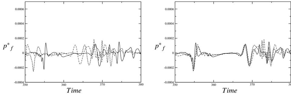
FIGURE 7. Adjoint pressure at three different locations at the centerline: at (dot-dashed)  $x = 8$ , (dashed)  $x = 9$ , and (solid)  $x = 10$ . When the actual evolutions of the variable (left) are shifted by the time corresponding to the convection velocity (right), there is an approximate superposition of the three lines, which indicates that these perturbations convect toward the nozzle at the convective speed.
