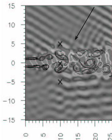
FIGURE 9. Adjoint pressure wave corresponding to far-field noise at an angle of  $60^\circ$  off the jet axis and at a frequency of  $St = 2.0$ . The Fourier transform of this field evaluated at the three points indicated is shown in Figure 10.
