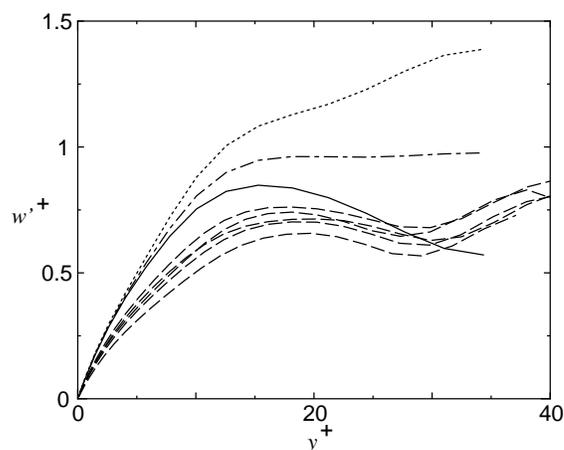
FIGURE 7. Spanwise rms velocities for the autonomous and the upper periodic solutions against  $y^+$ . ----, the autonomous solutions from table 1; —, the whole time average of the upper periodic solution with  $T_p^+ = 188$  in table 4. —, the time average of the upper periodic solution in a production phase  $P^+ > D^+$ ; ·····, the time average of the upper periodic solution in a dissipation phase  $P^+ < D^+$ .
