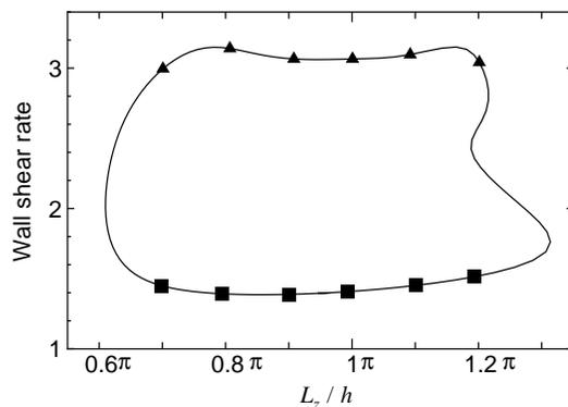
FIGURE 1. The dimensionless wall shear rate for Nagata's solution versus the spanwise period  $L_z$ . The Reynolds number  $Re$  and the streamwise period  $L_x$  are fixed as  $Re = 400$  and  $L_x = 2\pi h$ .
