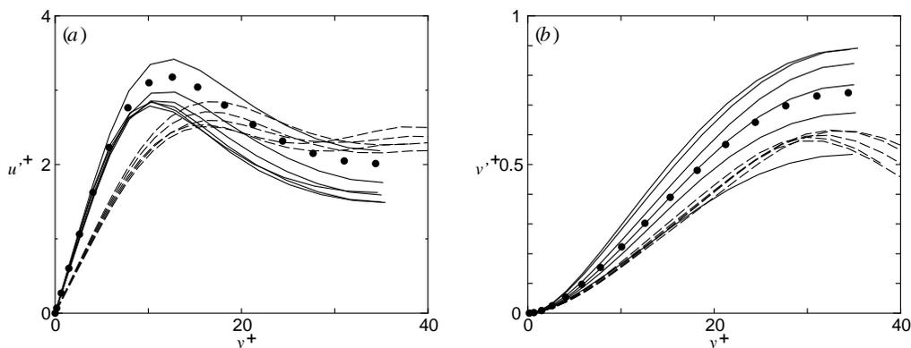
FIGURE 3. Rms velocities for the autonomous solutions, Nagata's upper branch, and the upper cycle versus  $y^+$ . (a) The streamwise component. (b) The wall-normal component. ----, the autonomous solutions from table 1; —, Nagata's upper-branch solutions from table 2; •, the upper cycle with the period  $T_p^+ = 188$  from table 4.
