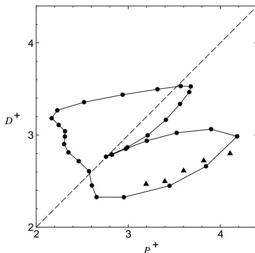
FIGURE 6. Total turbulent production and dissipation rates for the autonomous and the upper periodic solutions.  $\blacktriangle$ , autonomous solutions from table 1;  $\bullet$ —, the upper periodic solution with  $T_p^+ = 188$  in table 4. The production and dissipation are in balance on the dashed diagonal.
