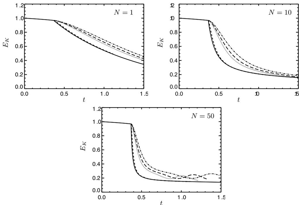
FIGURE 1. Evolution with time of the kinetic energy at different Stuart number and magnetic Reynolds number. — quasi-static approximation; - - - -  $R_m = 0.1$ ; .....  $R_m = 2$ ; - · - ·  $R_m = 3$ ; - - - -  $R_m = 5$ .
