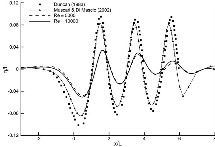
FIGURE 3. Submerged NACA 0012. Wave profiles for different Reynolds numbers.
