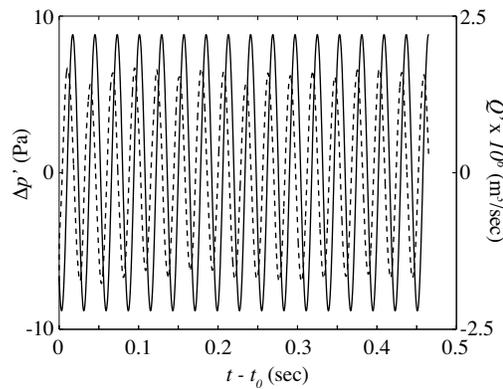
FIGURE 3. Fluctuations in aperture volume flow rate (—) and pressure drop (---) for forcing at 360 Hz.
