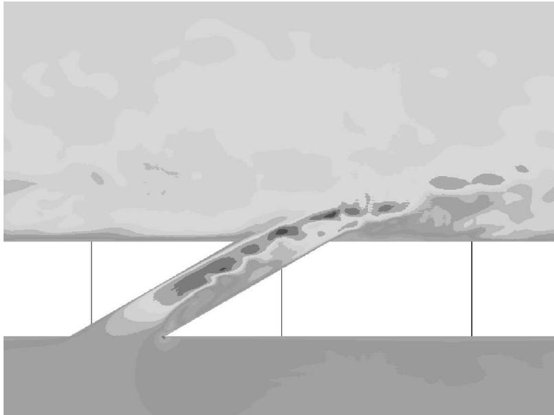
FIGURE 4. Snapshot of streamwise component of velocity from LES with 180 Hz forcing.
