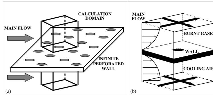
FIGURE 1. Adapted from Mendez *et al.* (2005): Numerical configuration of the multi-perforated liner. (a) Computational domain of single jet relative to the infinite array (b) Bi-periodic directions depicted with arrows, in domain extended equally above and below the aperture.
