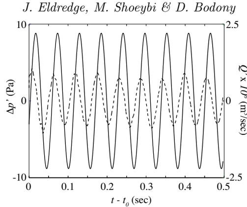
FIGURE 2. Fluctuations in aperture volume flow rate (—) and pressure drop (---) for forcing at 180 Hz. Time is measured relative to the instant of introduction of fluctuations.
