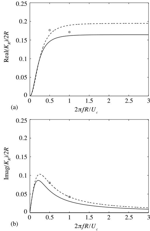
FIGURE 5. (a) Real and (b) imaginary components of Rayleigh conductivity of aperture. Modified Howe conductivity with  $t/R = 8$  (—); Modified Howe conductivity with  $t/R = 6.5$  (---); LES results (o).
